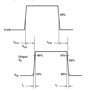
Fig. 10 Switching Times Definition for Inverters
