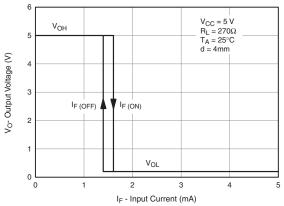
Fig. 2 Output Voltage vs. Input Current (Buffers)
