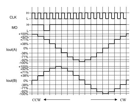
Note: MO signal is shown in the above timing chart when MO pin is connected with a pull-up resistor to VCC. Note: Timing charts may be simplified for explanatory purpose.
