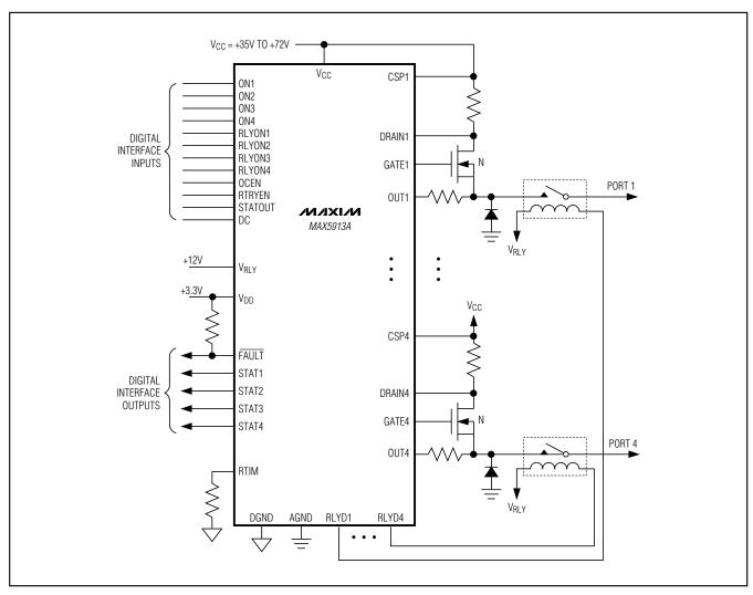
Figure 5. Typical Application Circuit
