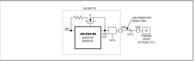
Figure 9. Power Sent Over Signal Pairs
