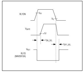
Figure 3. Port Turn-On Delay, Relay Turn-Off Delay
