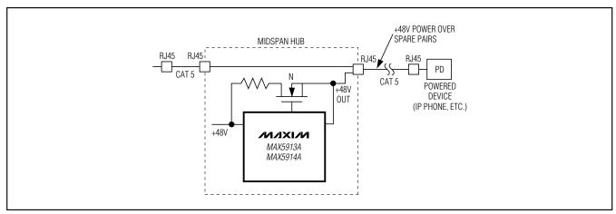
Figure 10. Power Sent Over Spare Pairs
