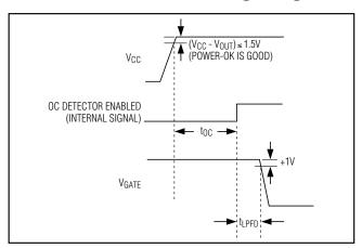
Figure 2. Open-Circuit Detector Deglitch Delay
