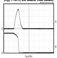
$ON = RLYON = V_{DD}$ ,  $R_L = 1\Omega$ ,  $R_{RTIM} = 2k\Omega$ A: I<sub>OUT</sub>, 5A/div B: VGATE, 20V/div
