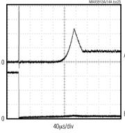
$0N = RLYON = V_{DD}, \ R_L = 1\Omega, \ R_{RTIM} = 2k\Omega$ A: I<sub>OUT</sub>, 200mA/div B: VGATE, 20V/div
