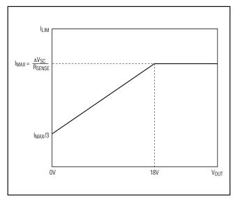
Figure 8. Foldback Current-Limit Response
