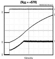
$RLYON = V_{DD}, \ R_L = 162\Omega, \ R_{RTIM} = 40 k\Omega, \ C_{LOAD} = 470 \mu F$
