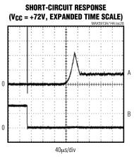
$\begin{array}{l} 0N = RLYON = V_{DD}, \, R_L = 1\Omega, \, R_{RTIM} = 2k\Omega \\ A: \, I_{OUT}, \, 200mA/div \\ B: \, V_{GATE}, \, 50V/div \end{array}$
