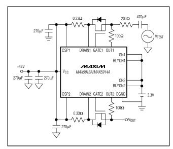
Figure 4. Channel-to-Channel Crosstalk Test Circuit
