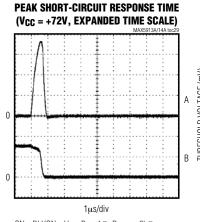
$ON=RLYON=V_{DD},\,R_L=1\Omega,\,R_{RTIM}=2k\Omega$  A:  $I_{OUT},\,5A/div$  B:  $V_{GATE},\,50V/div$
