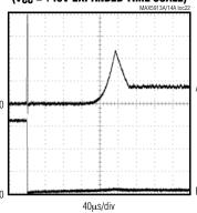
$0N = RLY0N = V_{DD}, \ R_L = 1\Omega, \ R_{RTIM} = 2k\Omega$ A: I<sub>OUT</sub>, 200mA/div B: V<sub>GATE</sub>, 20V/div
