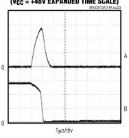
$0N = RLY0N = V_{DD}, \ R_L = 1\Omega, \ R_{RTIM} = 2k\Omega$ A: I<sub>OUT</sub>, 5A/div B: V<sub>GATE</sub>, 20V/div
