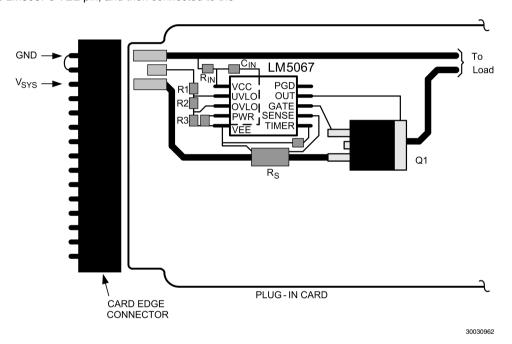
FIGURE 17. Suggested Board Connector Design
