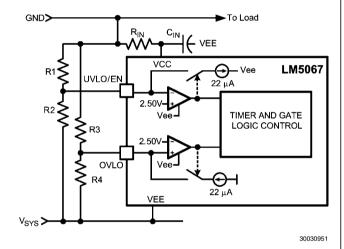
FIGURE 12. Programming the Four Thresholds
