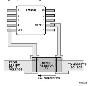
**FIGURE 7. Sense Resistor Connections**
