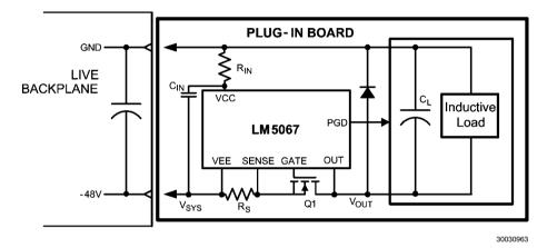
FIGURE 18. Output Diode Required for Inductive Loads
