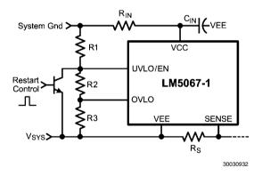
FIGURE 5. Latched Fault Restart Control
