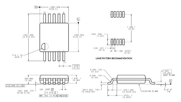
CONTROLLING DIMENSION IS INCH VALUES IN [] ARE MILLIMETERS DIMENSIONS IN ( ) FOR REFERENCE ONLY
