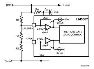
FIGURE 11. UVLO and OVLO Thresholds Set By R1-R3
