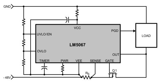
**Negative Power Bus In-Rush and Fault Protection**
