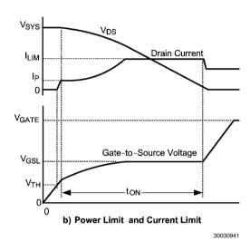
FIGURE 10. MOSFET Power Up Waveforms
