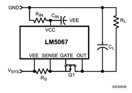
FIGURE 9. Load Draws Current During Turn-On
