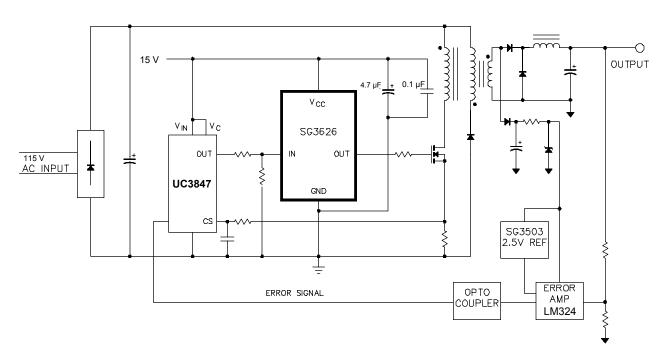
**Figure 15.**A low-impedance resistive divider network can also be used as the interface between the PWM high-voltage logic output and the SG3626 power driver. In this 200 kHz current mode converter, the UC3847 provides control, while the SG3626 provides high power drive and minimizes ground spiking in the control IC.
