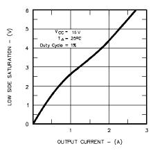
Figure 9 · Low Side Saturation vs. Output Current
