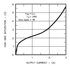
Figure 8 · High Side Saturation vs. Output Current
