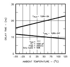
Figure 5 · Propagation Delay vs. Ambient Temperature
