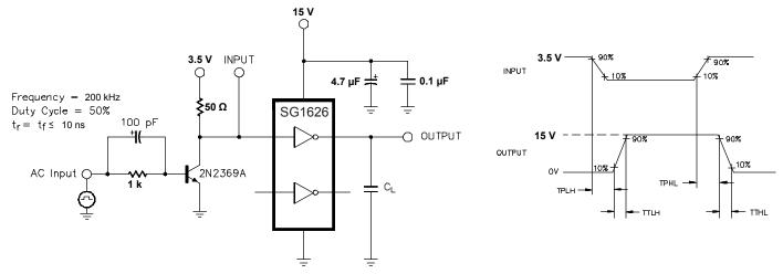
Figure 1 · AC Test Circuit and Switching Time Waveforms
