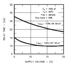
Figure 3 · Propagation Delay vs. Supply Voltage
