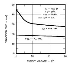
Figure 2 · Transition Times vs. Supply Voltage
