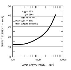
Figure 7 · Supply Current vs. Capacitive Load
