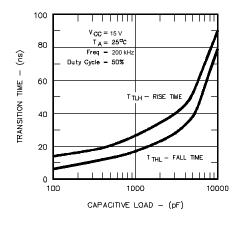
Figure 6  $\cdot$  Transition Times vs. Capacitive Load
