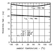
Figure 4 · Transition Times vs. Ambient Temperature
