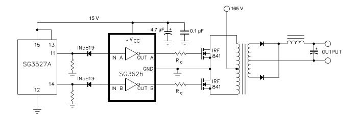
**Figure 12.**When the SG3626 is driven from a totem-pole source with a peak output greater than 6 V, a low-current, fast-switching blocking diode is required at each logic input for protection. In this push-pull converter, the inverted logic outputs of the 3527A are ideal control sources for the power driver.
