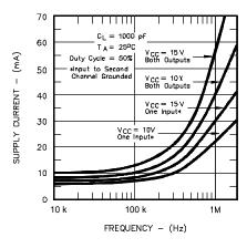
Figure 10 · Supply Current vs. Frequency
