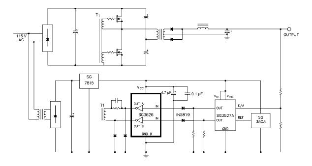
**Figure 14.**In half or full-bridge power supplies, driving the isolation transformers directly from the PWM can cause excessive IC temperatures, especially above 100 kHz. This circuit uses the high drive capacity of the SG3626 to solve the problem.
