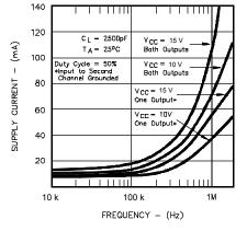
Figure 11 · Supply Current vs. Frequency
