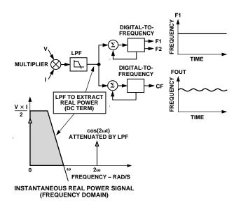
Figure 12. Real Power to Frequency Conversion
