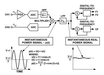
Figure 2. Signal Processing Block Diagram
