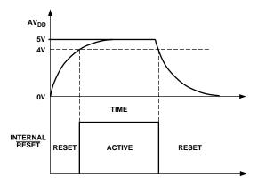
Figure 8. On-Chip Power Supply Monitor
