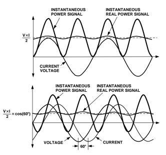
Figure 3. DC Component of Instantaneous Power Signal Conveys Real Power Information PF < 1
