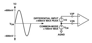
Figure 4. Maximum Signal Levels, Channel 2
