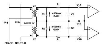
Figure 6. Typical Connection for Channel 1
