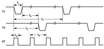
Figure 1. Timing Diagram for Frequency Outputs
