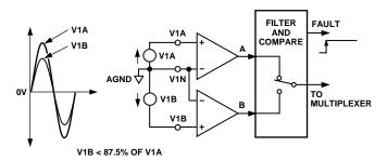
Figure 13. Fault Conditions for Inactive Input Less than Active Input
