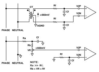
Figure 7. Typical Connections for Channel 2
