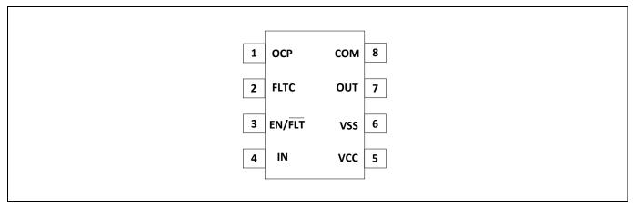
Figure 3 PG-DSO-8-70 (top view)
