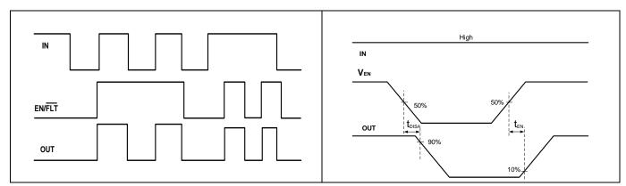
Figure 13 Input/output/enable pins timing diagram Figure 14 EN pin switching time waveform
