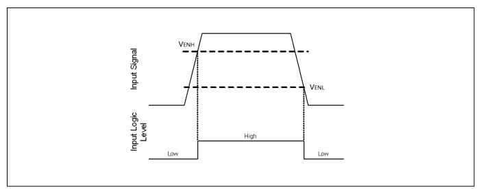
Figure 15 EN input thresholds
