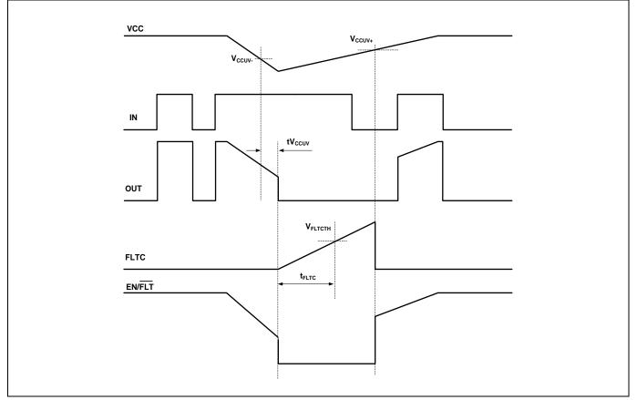
Figure 9 Vcc under voltage protection waveform definitions two
