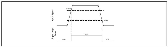
Figure 7 IN input thresholds
