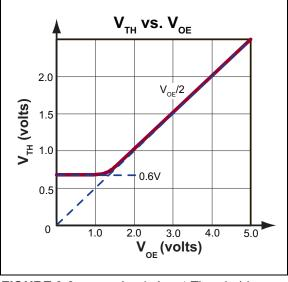
FIGURE 3-2: Logic Input Threshold.
