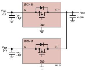
Figure 1. Redundant Diode-OR Power Supplies
