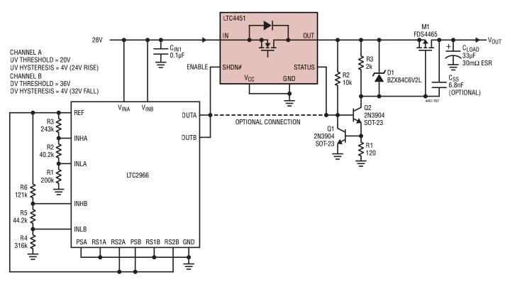
Figure 7. 28V Output Disconnect Switch Controlled by LTC2966
