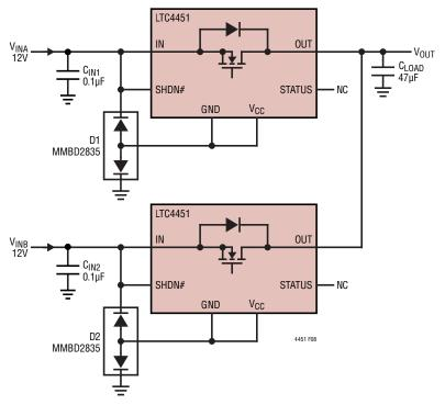
Figure 8. 12V Diode-OR with Reverse Input Voltage Protection
