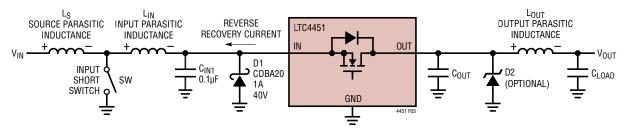
Figure 3. Input Short Protection Circuit with Parasitic Inductances
