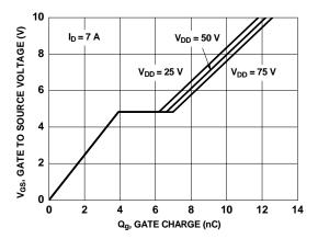
Figure 7. Gate Charge Characteristics
