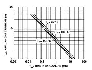
Figure 9. Unclamped Inductive Switching Capability
