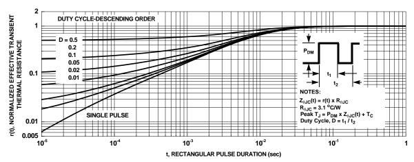
Figure 13. Junction-to-Case Transient Thermal Response Curve
