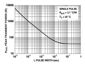
Figure 12. Single Pulse Maximum Power Dissipation
