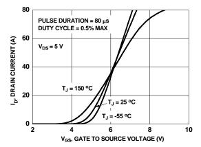
Figure 5. Transfer Characteristics
