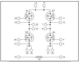
All multiple inputs and outputs must be shorted together Example: 13/14; 29/30; 22/23 ...
