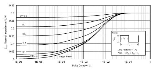
Figure 12 • Maximum Transient Thermal Impedance
