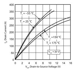
Figure 1 • Drain Current vs. V<sub>DS</sub>
