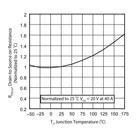
Figure 5 • RDS(on) vs. Junction Temperature
