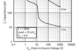
Figure 7 • Capacitance vs. Drain-to-Source Voltage
