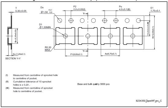
Figure 22: PowerFLAT™ 5x6 package orientation in carrier tape
