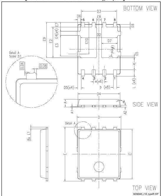
Table 8: PowerFLAT™ 5x6 double island WF type R mechanical data
