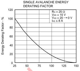
Starting Ton - Starting Channel Temperature - °C
