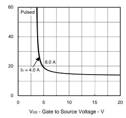
RDS(m) - Drain to Source On-state Resistance - mΩ
