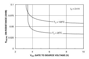
Figure 4. On-Resistance Variation with Gate-to-Source Voltage.
