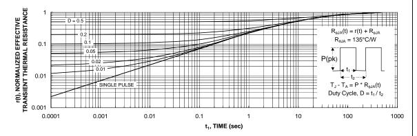
Figure 11. Transient Thermal Response Curve.
