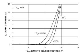
Figure 5. Transfer Characteristics.
