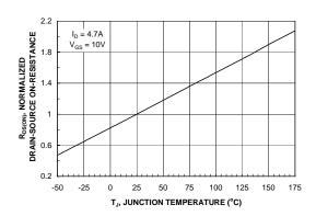
Figure 3. On-Resistance Variation with Temperature.
