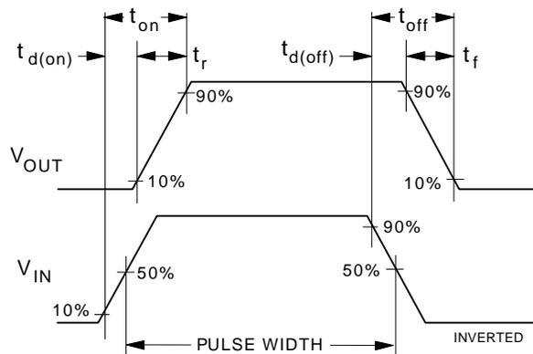
Figure 12. Switching Waveforms.
