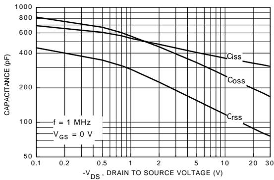
Figure 9. Capacitance Characteristics.
