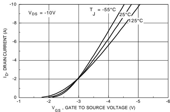
Figure 5. Transfer Characteristics.
