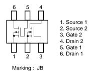
The diode connected between the gate and source of the transistor serves as a protector against ESD. When this device is actually used, an additional protection circuit is externally required if a voltage exceeding the rated voltage may be applied to this device.
