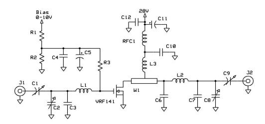
C1, 2, 8, 9 - ARCO 463 C3 C7 - 25 pF ATC 100B C4 C10 C12 - 0.1uF 100V SMT C5 - 1 uF 15WV tant C6 - 270 pF ATC 100B C10 - .05 100V 1206 SMT C11 - 15uF 100V Elect
