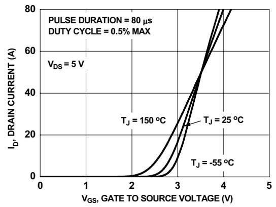
Figure 5. Transfer Characteristics
