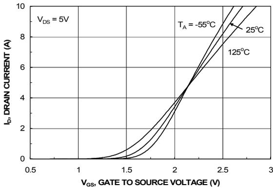
Figure 5. Transfer Characteristics
