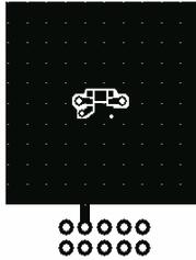
a)  $70^\circ\text{C/W}$  when mounted on a  $1\text{in}^2$  pad of 2 oz copper
