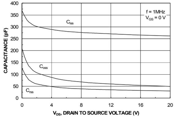
Figure 8. Capacitance Characteristics
