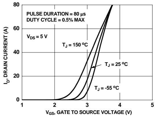
**Figure 5. Transfer Characteristics**
