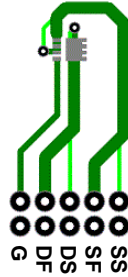
b) 125^\circ\text{C/W} when mounted on a minimum pad
