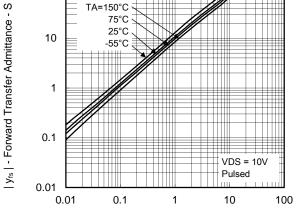
FORWARD TRANSFER ADMITTANCE vs. DRAIN
