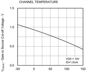
GATE TO SOURCE CUT-OFF VOLTAGE vs.
