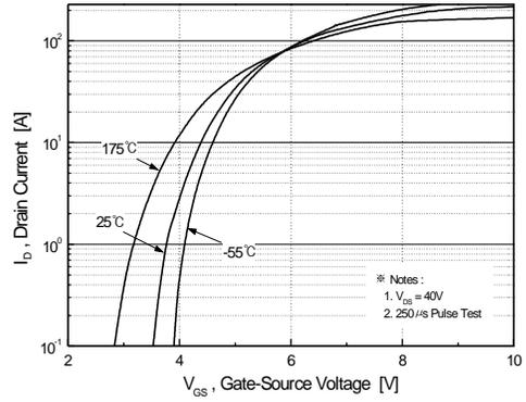
**Figure 2. Transfer Characteristics**
