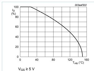
Fig. 1. Normalized continuous drain current as a function of solder point temperature
