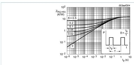
Fig. 5. Transient thermal impedance from junction to solder point as a function of pulse duration
