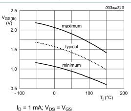
Fig. 11. Gate-source threshold voltage as a function of junction temperature
