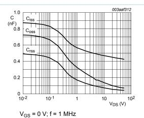
Fig. 13. Input, output and reverse transfer capacitances as a function of drain-source voltage; typical
