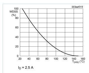
Fig. 3. Normalised drain-source non-repetitive avalanche energy as a function of mounting-base temperature
