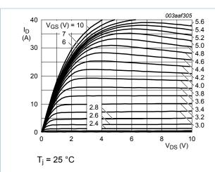
Output characteristics: drain current as a
