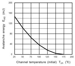
Fig. 8.15 E<sub>AS</sub> - T<sub>ch</sub>(Guaranteed Maximum)
