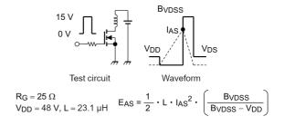
Fig. 8.16 Test Circuit/Waveform
