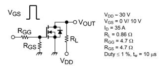
Fig. 6.2.1 Switching Time Test Circuit
