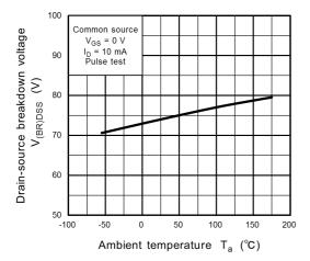
Fig. 8.11 V<sub>(BR)DSS</sub> - T<sub>a</sub>
