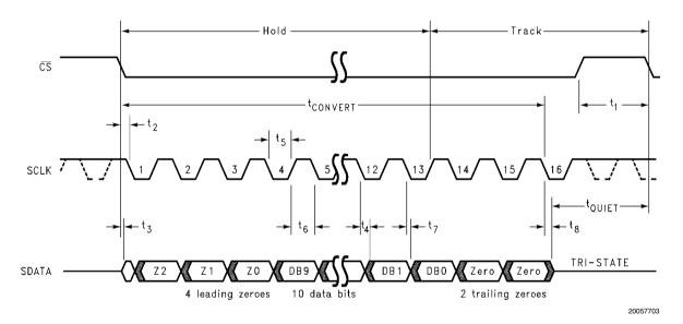
FIGURE 2. ADCS7477 Serial Interface Timing Diagram
