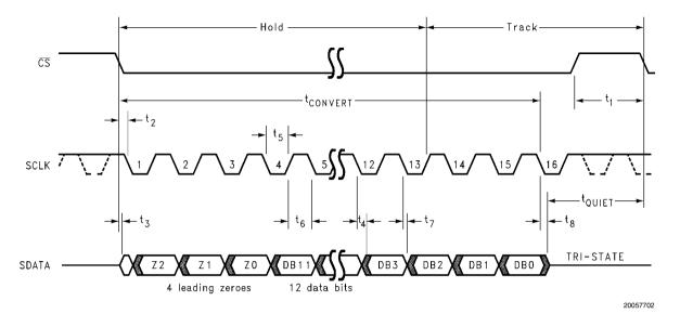
FIGURE 1. ADCS7476 Serial Interface Timing Diagram
