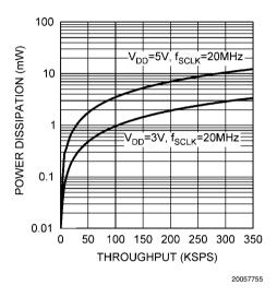
FIGURE 12. Maximum Power Consumption vs. Throughput
