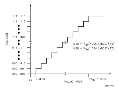
FIGURE 6. ADCS7476/77 Ideal Transfer Characteristic
