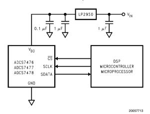
FIGURE 8. Typical Application Circuit
