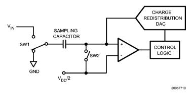
FIGURE 5. ADCS7476/77/78 in Hold Mode
