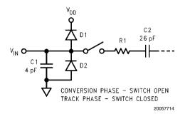
FIGURE 9. Equivalent Input Circuit
