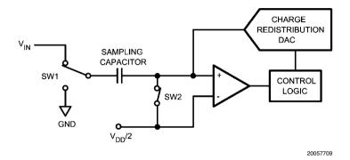
FIGURE 4. ADCS7476/77/78 in Track Mode
