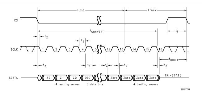
FIGURE 3. ADCS7478 Serial Interface Timing Diagram
