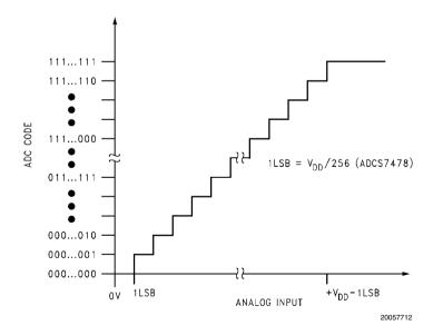
FIGURE 7. ADCS7478 Ideal Transfer Characteristic
