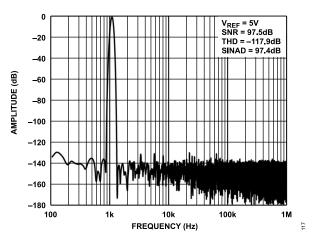
Figure 15. 1 kHz, -0.5 dBFS Input Tone FFT, Wide View, Differential, G = 0.909,  $V_{REF} = 5$  V, Low Power Mode
