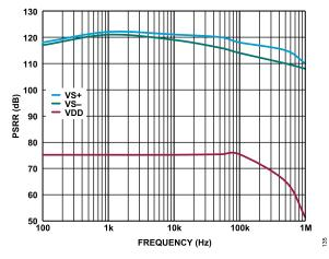
Figure 33. PSRR vs. Frequency
