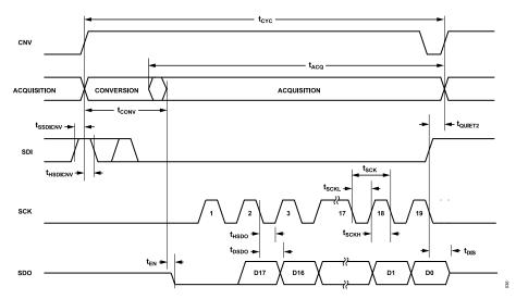
Figure 67. CS Mode, 4-Wire with Busy Indicator Serial Interface Timing Diagram
