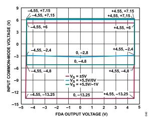
Figure 36. Input Common-Mode Voltage vs. FDA Output Voltage, G = 0.909, Differential Input
