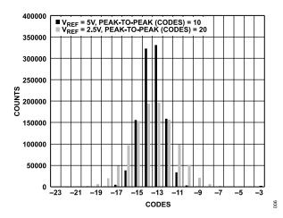
Figure 10. Histogram of a DC Input at the Code Transition,  $V_{REF}$  = 2.5 V and  $V_{REF}$  = 5 V
