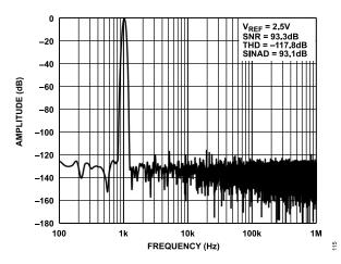
Figure 13. 1 kHz, -0.5 dBFS Input Tone FFT, Wide View, G = 1,  $V_{REF}$  = 2.5 V, Differential
