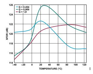
Figure 26. SFDR vs. Temperature for G = 0.454, G = 0.909, and G = 1.9,  $f_{\rm IN}$  = 1kHz
