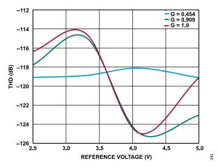
Figure 22. THD vs. Reference Voltage, G = 0.454, G = 0.909, and G = 1.9,  $f_{IN} = 1 \text{ kHz}$
