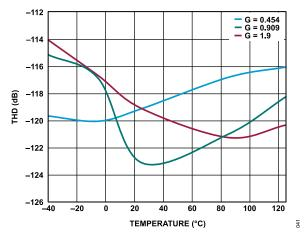
Figure 23. THD vs. Temperature for G = 0.454, G = 0.909, and G = 1.9,  $f_{\rm IN}$  = 1 kHz
