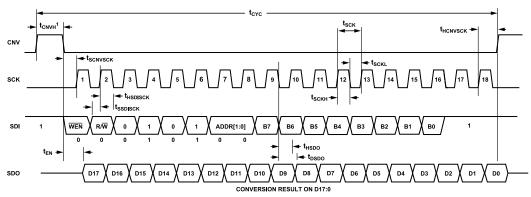
Figure 52. Register Read Timing Diagram
