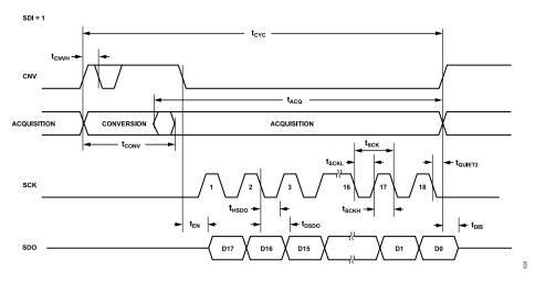
Figure 59. CS Mode, 3-Wire Without Busy Indicator Serial Interface Timing Diagram (SDI High)
