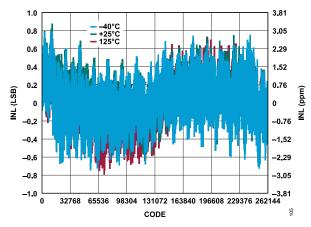
Figure 5. INL vs. Code for Various Temperatures, V<sub>REF</sub> = 5 V, G = 0.454
