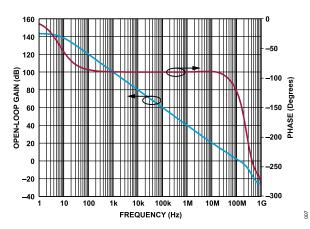
Figure 6. ADC Driver Open-Loop Gain and Phase vs. Frequency
