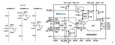
Figure 48. Differential Configuration with G = 1.9
