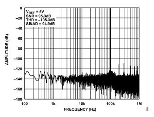
Figure 16. 100 kHz, -0.5 dBFS Input Tone FFT, Wide View, G = 1, V<sub>REF</sub> = 5 V
