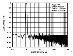
Figure 11. 1 kHz, -0.5 dBFS Input Tone Fast Fourier Transform (FFT), Wide View, G = 1,V<sub>REF</sub> = 5 V, Differential
