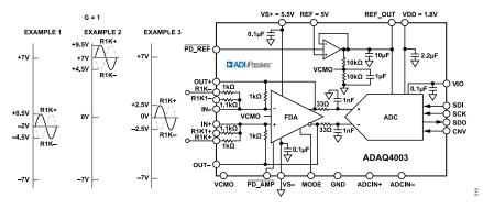
Figure 47. Differential Configuration with G = 1
