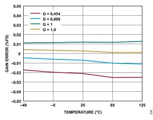
Figure 30. Gain Error vs. Temperature, V<sub>REF</sub> = 5.0 V, Normal Mode
