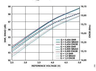
Figure 18. SNR, SINAD, and Effective Number of Bits (ENOB) vs. Reference Voltage for G = 0.454, G = 0.909, and G = 1.9, f<sub>IN</sub> = 1 kHz
