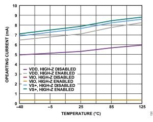
Figure 29. Operating Current vs. Temperature, 2 MSPS
