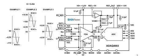
Figure 45. Differential Configuration with G = 0.454
