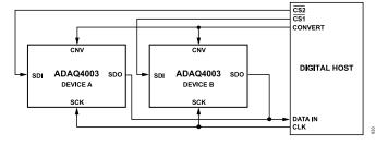
Figure 64. CS Mode, 4-Wire Without Busy Indicator Connection Diagram
