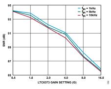
Figure 49. SNR vs. LTC6373 Gain Setting, LTC6373 Driving the ADAQ4003 (Gain = 0.454)
