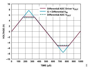
Figure 39. Output Drive Recovery, f<sub>IN</sub> = 1 kHz
