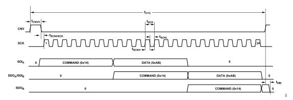
Figure 54. Register Write Timing Diagram, Daisy-Chain Mode
