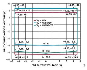
Figure 35. Input Common-Mode Voltage vs. FDA Output Voltage, G = 0.454, Differential Input
