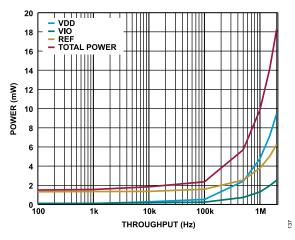
Figure 32. Power vs. Throughput
