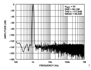
Figure 12. 1 kHz, -0.5 dBFS Input Tone FFT, Wide View, G = 1,  $V_{REF}$  = 5 V, Single-Ended
