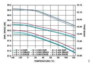
Figure 19. SNR, SINAD, and ENOB vs. Temperature, G =1.9, G = 0.909, and G = 0.454,  $f_{\rm IN}$  = 1 kHz
