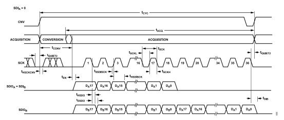
Figure 69. Daisy-Chain Mode Serial Interface Timing Diagram
