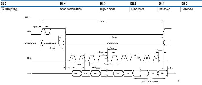
Figure 55. CS Mode, 3-Wire Without Busy Indicator Serial Interface Timing Diagram Including Status Bits (SDI High)
