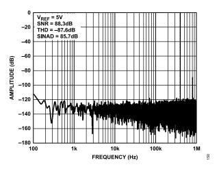
Figure 20. 400 kHz, -0.5 dBFS Input Tone FFT, G = 1, Wide View, V<sub>REF</sub> = 5 V
