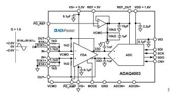
Figure 44. Single-Ended to Differential Configuration with G = 1.9
