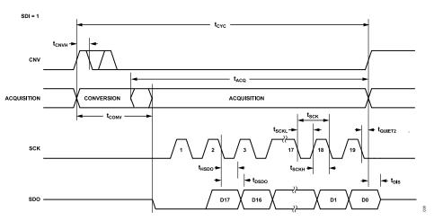
Figure 61. CS Mode, 3-Wire with Busy Indicator Serial Interface Timing Diagram (SDI High)
