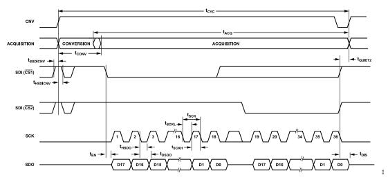
Figure 65. CS Mode, 4-Wire Without Busy Indicator Serial Interface Timing Diagram
