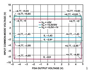
Figure 37. Input Common-Mode Voltage vs. FDA Output Voltage, G = 1.9, Differential Input
