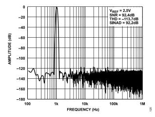
Figure 17. 1 kHz, -0.5 dBFS Input Tone FFT, Wide View, Differential, G = 0.909, V<sub>REF</sub> = 2.5 V, Low Power Mode
