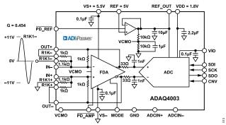
Figure 41. Single-Ended to Differential Configuration with G = 0.454
