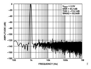
Figure 14. 1 kHz, -0.5 dBFS Input Tone FFT, Wide View, G = 1,  $V_{REF}$  = 2.5 V, Single-Ended
