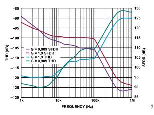
Figure 24. THD and SFDR vs. Frequency for G = 0.909 and G = 1.9,  $V_{REF}$  = 5 V
