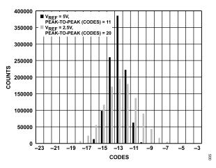
Figure 9. Histogram of a DC Input at the Code Center,  $V_{REF}$  = 2.5 V and  $V_{REF}$  = 5 V
