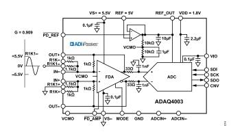
Figure 42. Single-Ended to Differential Configuration with G = 0.909
