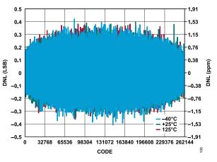
Figure 8. DNL vs. Code for Various Temperatures, V<sub>REF</sub> = 5 V, G = 0.454
