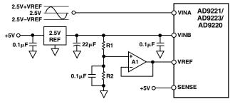
Figure 24. External Reference –  $V_{CM}$  = 2.5 V (2.5 V on VINB, Resistor Divider to Make VREF)
