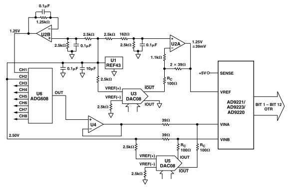
Figure 35. Typical Multichannel Data Acquisition System
