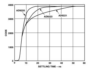
Figure 3. Settling Time
