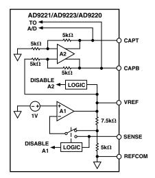
Figure 9. Equivalent Reference Circuit
