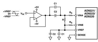
Figure 15. AC-Coupled Input
