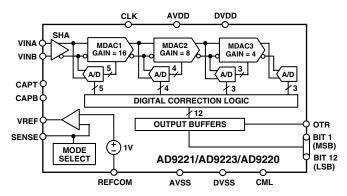
amplifier (SHA) is equally suited for both multiplexed systems that switch full-scale voltage levels in successive channels as well as sampling single-channel inputs at frequencies up to and beyond the Nyquist rate. Also, the AD9221/AD9223/AD9220 is well suited for communication systems employing Direct-IF down conversion since the SHA in the differential input mode can achieve excellent dynamic performance *far beyond* its specified Nyquist frequency.<sup>2</sup>
