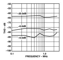
TPC 5. THD vs. Input Frequency (Input Span = 2.0 V p-p,  $V_{CM}$  = 2.5 V)
