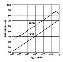
TPC 18. SNR/SFDR vs.  $A_{IN}$  (Input Amplitude) ( $f_{IN} = 1.5$  MHz, Input Span = 2 V p-p,  $V_{CM} = 2.5$  V)
