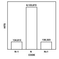
TPC 21. "Grounded-Input" Histogram (Input Span = 2 V p-p)
