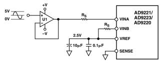
Figure 13. Single-Ended AD9221/AD9223/AD9220 Op Amp Drive Circuit
