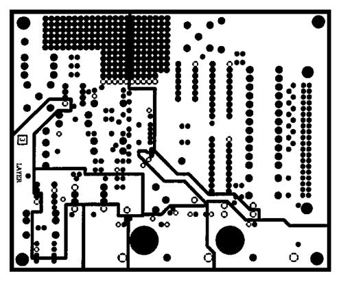
Figure 40. Evaluation Board Power Plane Layout
