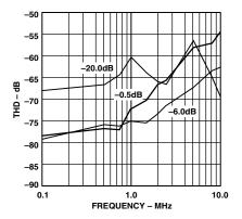
TPC 25. THD vs. Input Frequency (Input Span = 5.0 V p-p,  $V_{CM}$  = 2.5 V)
