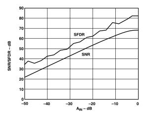
Figure 34. AD9220 Differential Input SNR/SFDR vs. Input Amplitude (A<sub>IN</sub>) @ 21.4 MHz
