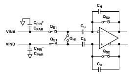
Figure 5. AD9221/AD9223/AD9220 Simplified Input Circuit
