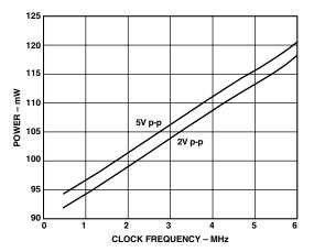
Figure 29b. AD9223 Power Consumption vs. Clock Frequency
