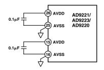
Figure 30. Analog Supply Decoupling
