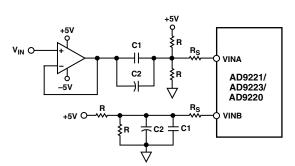
Figure 16. AC-Coupled Input-Flexible Input Span,  $V_{CM} = 2 V$
