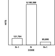
TPC 3. "Grounded-Input" Histogram (Input Span = 2 V p-p)
