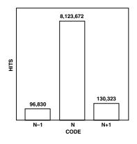
TPC 12. "Grounded-Input" Histogram (Input Span = 2 V p-p)
