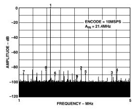
Figure 33. IF Sampling a 21.4 MHz Input Using the AD9220 ( $V_{CM} = 2.5 V$ , Input Span = 2 V p-p)
