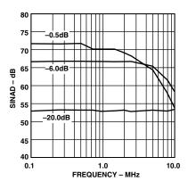
TPC 15. SINAD vs. Input Frequency (Input Span = 5.0 V p-p,  $V_{CM}$  = 2.5 V)
