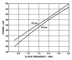
Figure 29a. AD9221 Power Consumption vs. Clock Frequency
