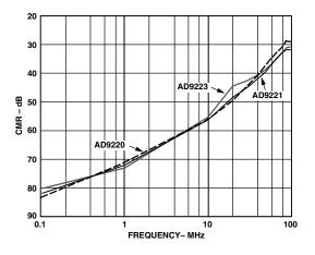
Figure 11. AD9221/AD9223/AD9220 Input CMR vs. Input Frequency
