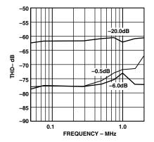
TPC 7. THD vs. Input Frequency (Input Span = 5.0 V p-p,  $V_{CM}$  = 2.5 V)
