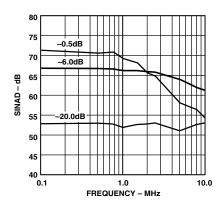
TPC 24. SINAD vs. Input Frequency (Input Span = 5.0 V p-p,  $V_{CM}$  = 2.5 V)
