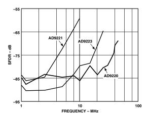
Figure 18. AD9221/AD9223/AD9220 SFDR vs. Input Frequency ( $V_{CM} = 2.5 V$ , 2 V p-p Input Span,  $A_{IN} = -0.5 dB$ )
