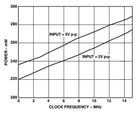
Figure 29c. AD9220 Power Consumption vs. Clock Frequency
