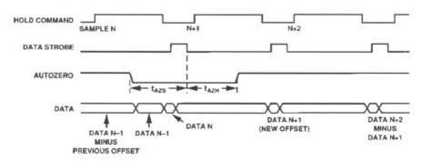
Figure 24. Autozero Cycle Operation
