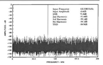
Figure 20. Full-Scale Power Spectral Density after Power-up at  $T_{CASE} = \pm 25^{\circ} C$  Without Calibration,  $\pm 5$  V Range, 16384-Point FFT, 500 kHz Sample Rate. Compare with Figure 4.
