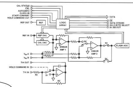
Figure 13. AD1385 Functional Block Diagram
