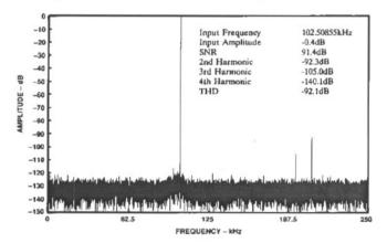
Figure 22. Same as Figure 21 Following Recalibration at  $T_{CASF} = +125^{\circ}C$
