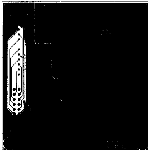
Figure 13d. Suggested Evaluation Circuit Board Solder Side Layout
