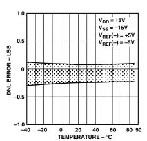
Figure 5. Typical DNL Error vs. Temperature
