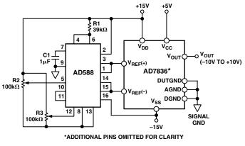
Figure 12. Bipolar ±5 V Operation
