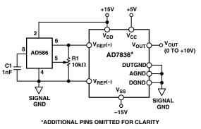
Figure 11. Unipolar +5 V Operation
