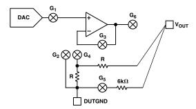
Figure 17. Output Stage Powering Up with CLR High While V<sub>DD</sub>/V<sub>SS</sub> < ±10 V
