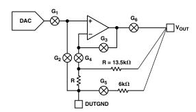
Figure 13. Block Diagram of AD7836 Output Stage
