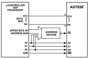
\*ADDITIONAL PINS OMITTED FOR CLARITY Figure 19. AD7836 Parallel Interface
