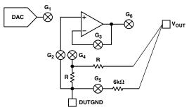
Figure 14. Output Stage with  $V_{DD} < 10 V$
