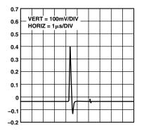
Figure 8. Typical Digital/Analog Glitch Impulse
