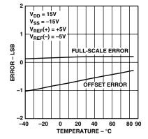
Figure 6. Offset and Full-Scale Error vs. Temperature
