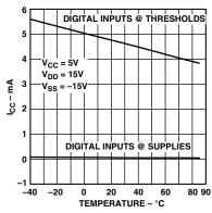
Figure 7. I<sub>CC</sub> vs. Temperature
