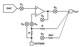
Figure 18. Output Stage Powering Up with  $\overline{CLR}$  High When  $V_{DD}/V_{SS}$  >  $\pm\,10$  V
