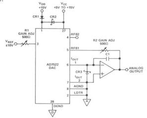
Figure 3. Unipolar Binary Operation (2-Quadrant Multiplication)
