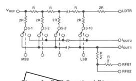
Figure 1. DAC Functional Diagram
