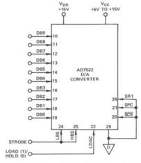
Figure 5. Single Byte Parallel Loading
