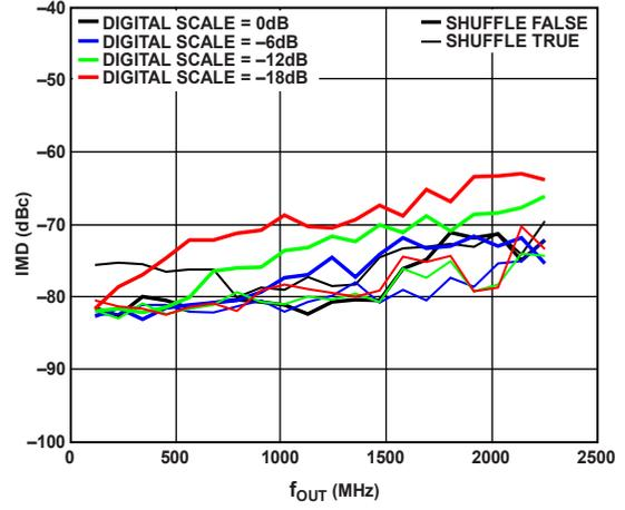
Figure 21. IMD vs.  $f_{OUT}$  over Digital Scale
