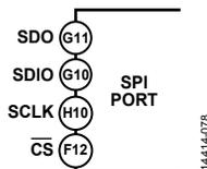
Figure 86. Serial Port Interface Pins (169-Ball CSP\_BGA)
