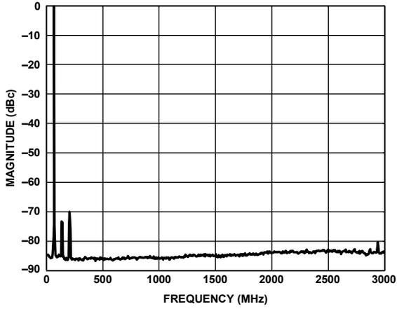
Figure 60. Single Carrier at 70 MHz Output
