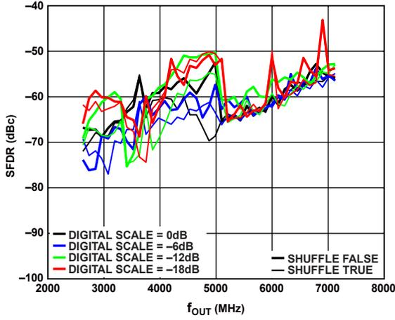
Figure 48. SFDR vs.  $f_{OUT}$  over Digital Scale
