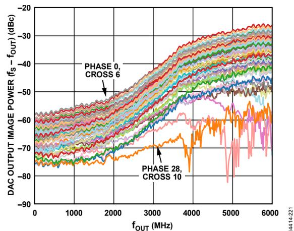
Figure 134. Performance Improvement from Tuning the Clock Input
