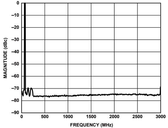
Figure 64. Four Carriers at 70 MHz Output (Shuffle On)
