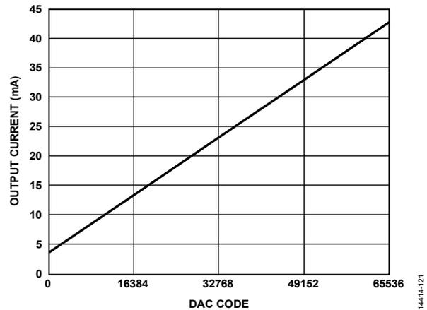
Figure 138. Gain Curve for ANA\_FULL\_SCALE\_CURRENT[9:0] = 1023, DAC Offset = 3.8 mA
