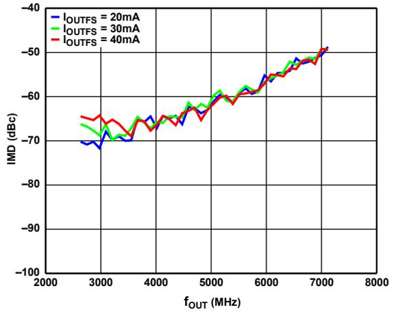
Figure 52. IMD vs.  $f_{OUT}$  over DAC  $I_{OUTFS}$
