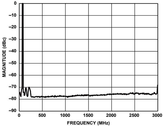
Figure 61. Four Carriers at 70 MHz Output
