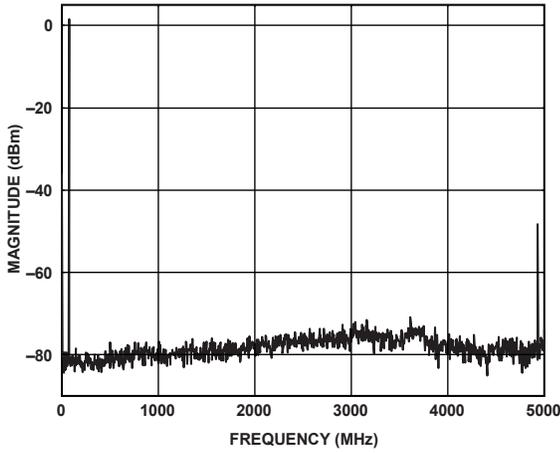
Figure 12. Single-Tone Spectrum at  $f_{OUT} = 70\text{ MHz}$
