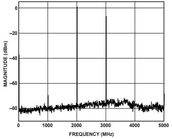
Figure 15. Single-Tone Spectrum at  $f_{OUT} = 2000\text{ MHz}$
