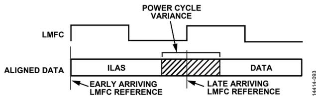
Figure 103. Link Delay > LMFC Period Example
