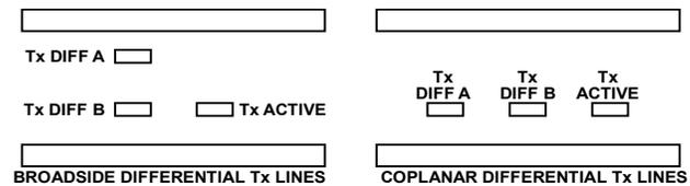
Figure 125. Broadside vs. Coplanar Differential Stripline Routing Techniques
