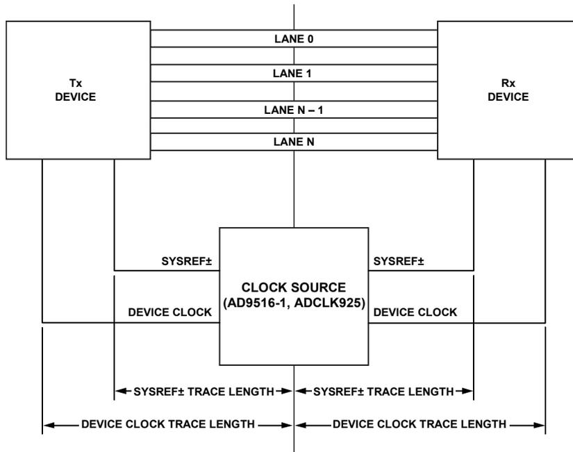
Figure 127. SYSREF± Signal and Device Clock Trace Length
