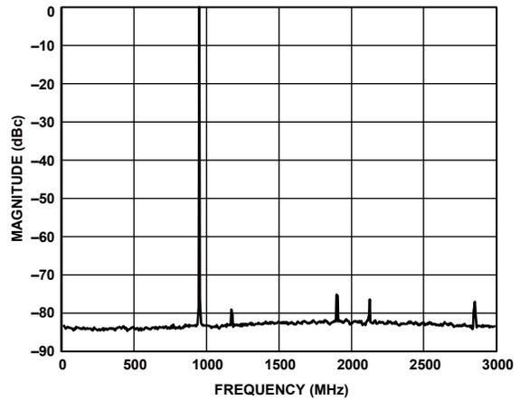
Figure 69. Single Carrier at 950 MHz Output (Shuffle On)
