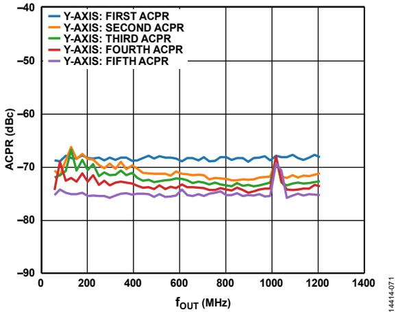
Figure 79. Four-Carrier ACPR vs.  $f_{OUT}$
