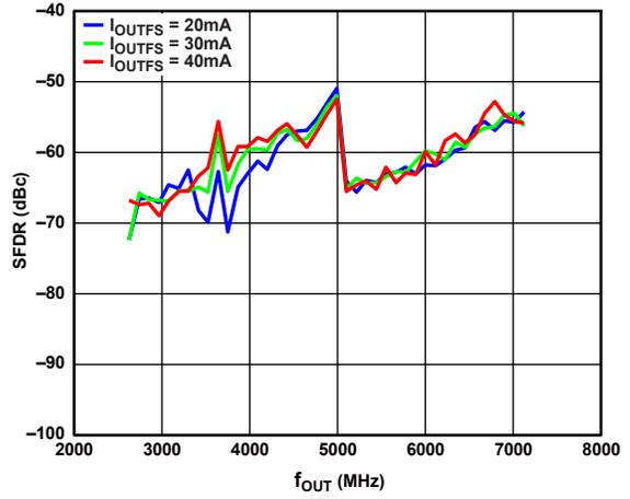
Figure 51. SFDR vs.  $f_{OUT}$  over DAC  $I_{OUTFS}$
