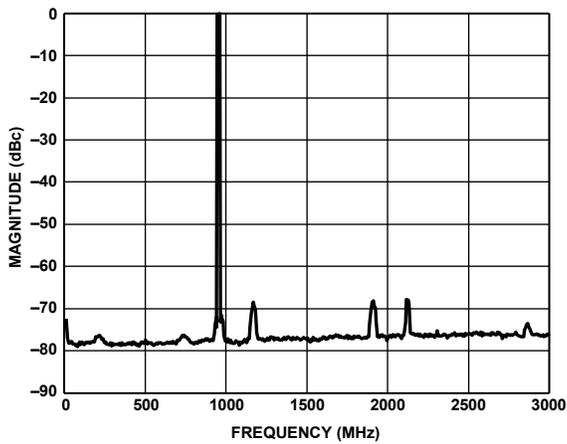
Figure 67. Four Carriers at 950 MHz Output
