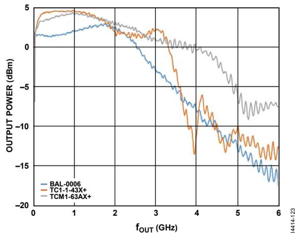
Figure 139. Measured DAC Output Response;  $f_{DAC} = 6$  GSPS
