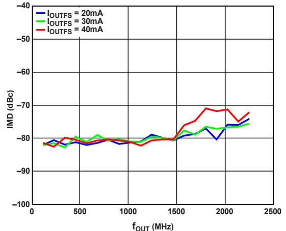
Figure 23. IMD vs.  $f_{OUT}$  over DAC  $I_{OUTFS}$
