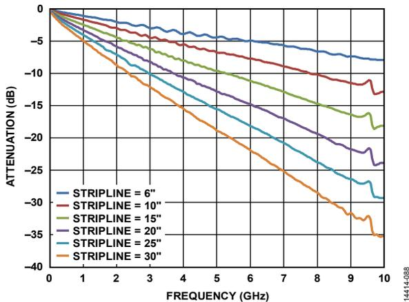
Figure 96. Insertion Loss of 50 Ohm Striplines on FR4
