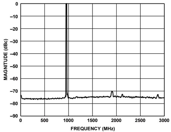
Figure 70. Four Carriers at 950 MHz Output (Shuffle On)
