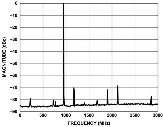
Figure 66. Single Carrier at 950 MHz Output
