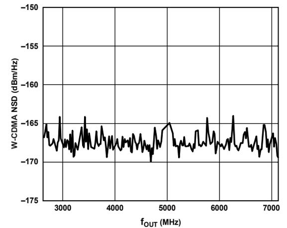
Figure 47. W-CDMA NSD vs.  $f_{OUT}$
