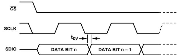
Figure 89. Timing Diagram for Serial Port Register Read
