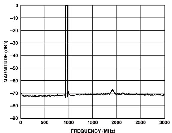
Figure 71. Eight Carriers at 950 MHz Output (Shuffle On)
