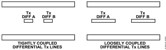
Figure 126. Tightly Coupled vs. Loosely Coupled Differential Traces
