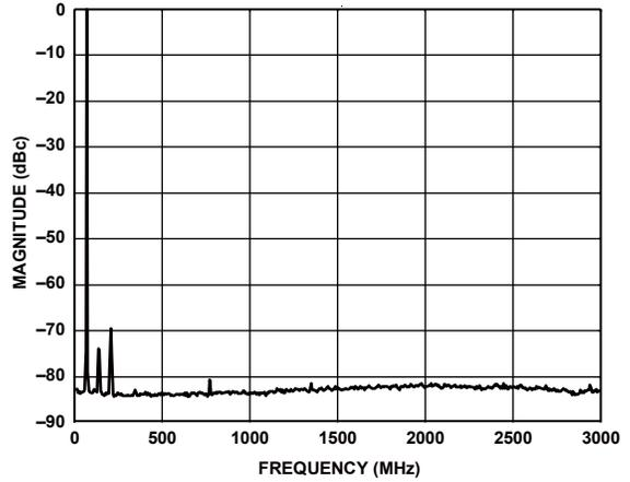
Figure 63. Single Carrier at 70 MHz Output (Shuffle On)
