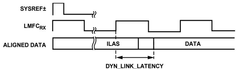
Figure 106. DYN\_LINK\_LATENCY\_x Illustration
