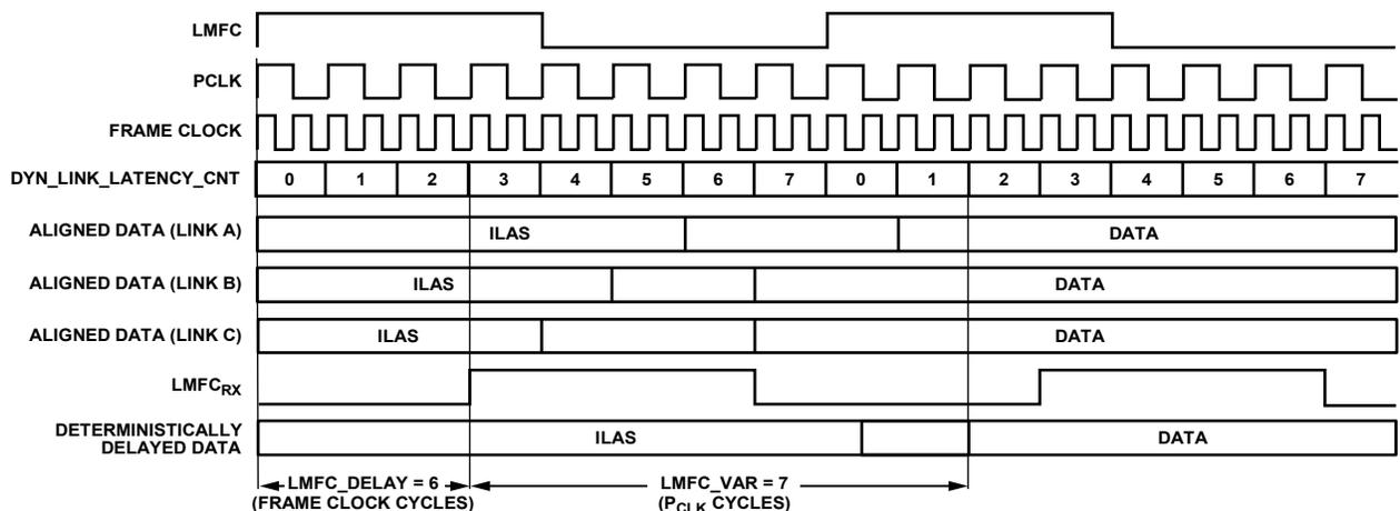
Figure 107. Multilink Synchronization Settings, Derived Method Example
