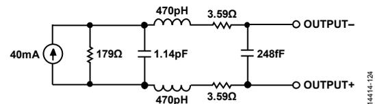
Figure 141. Equivalent Circuit Model of the DAC Output
