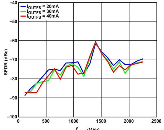
Figure 22. SFDR vs.  $f_{OUT}$  over DAC  $I_{OUTFS}$
