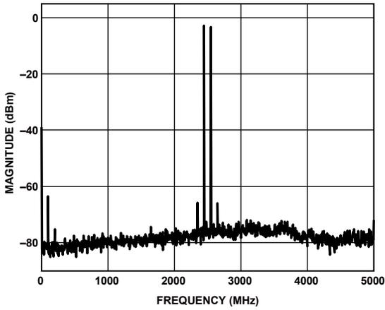
Figure 42. Single-Tone Spectrum at  $f_{OUT} = 2350\text{ MHz}$
