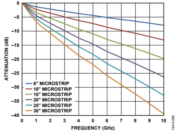
Figure 97. Insertion Loss of 50 Ohm Microstrips on FR4
