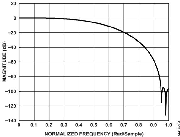
Figure 118. Fourth 2x Half-Band 11.25% Filter Response
