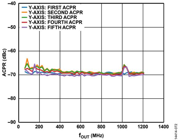
Figure 80. Eight-Carrier ACPR vs.  $f_{OUT}$
