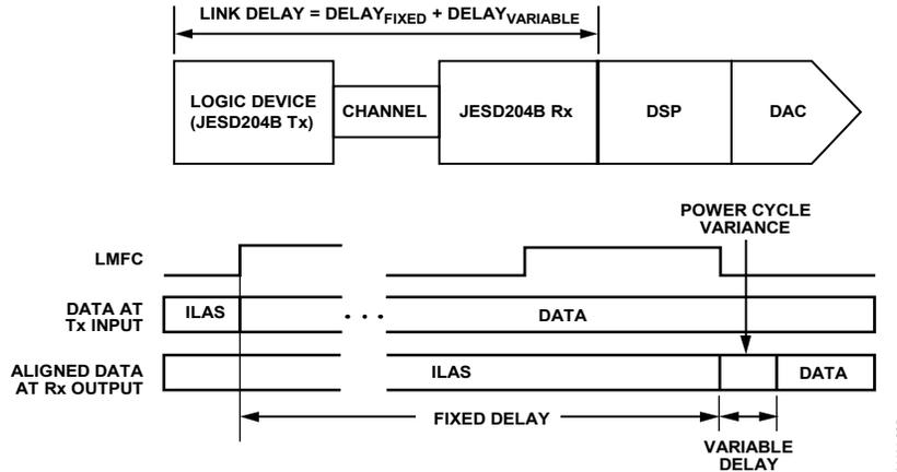
Figure 102. JESD204B Link Delay = Fixed Delay + Variable Delay
