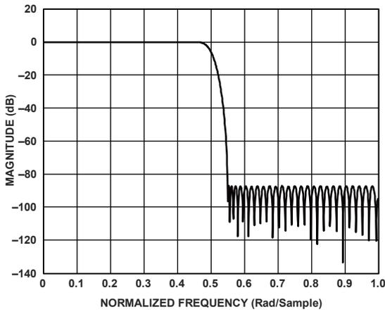
Figure 113. First 2x Half-Band 90% Filter Response
