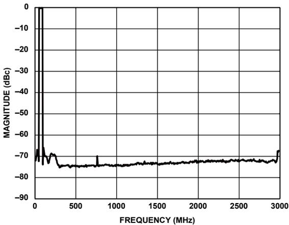
Figure 62. Eight Carriers at 70 MHz Output
