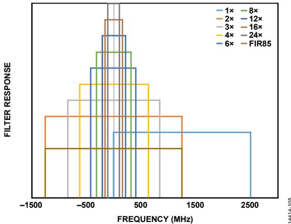
Figure 110. All Band Responses of Interpolation Filters
