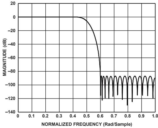
Figure 112. First 2x Half-Band 80% Filter Response
