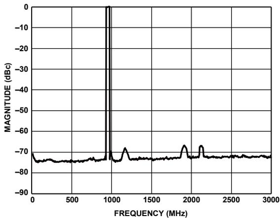
Figure 68. Eight Carriers at 950 MHz Output
