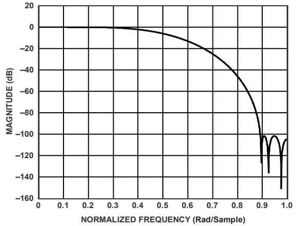
Figure 117. Third 2x Half-Band 22.5% Filter Response
