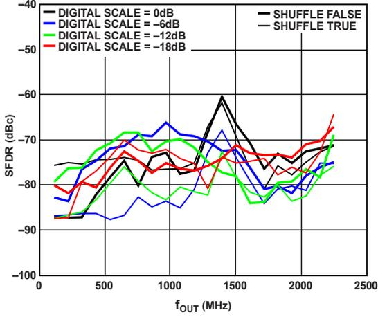
Figure 18. SFDR vs.  $f_{OUT}$  over Digital Scale
