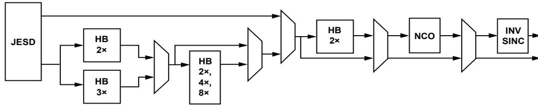
Figure 109. Block Diagram of the Main Digital Datapath
