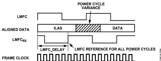
Figure 104. LMFC\_DELAY\_x to Compensate for Link Delay > LMFC
