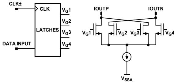
Figure 128. Quad-Switch Architecture
