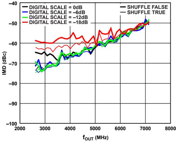
Figure 49. IMD vs.  $f_{OUT}$  over Digital Scale
