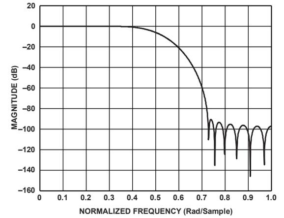
Figure 116. Second 2x Half-Band 45% Filter Response
