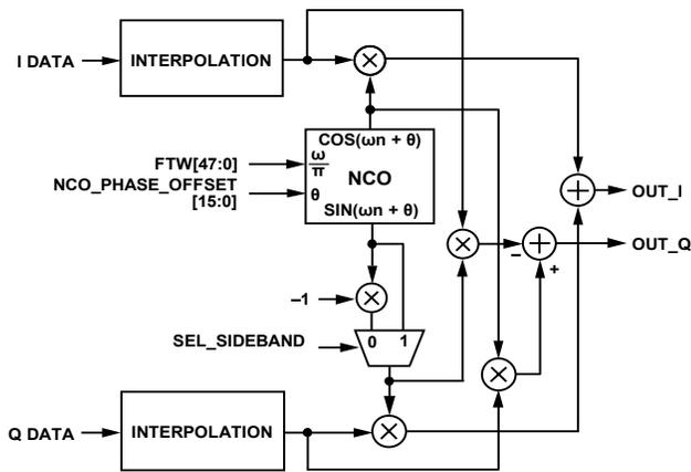
Figure 120. NCO Modulator Block Diagram
