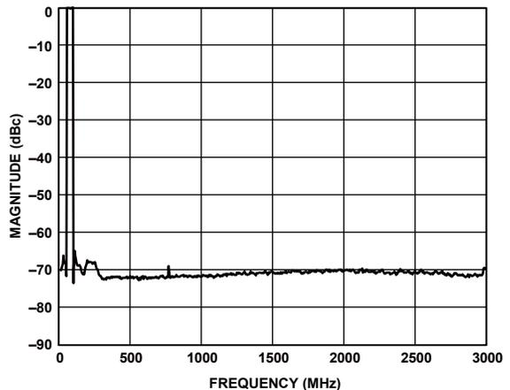
Figure 65. Eight Carriers at 70 MHz Output (Shuffle On)
