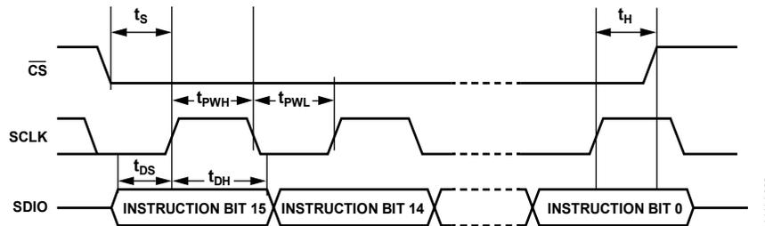
Figure 90. Timing Diagram for Serial Port Register Write
