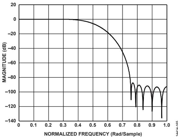
Figure 119. FIR85 2x Half-Band 45% Filter Response
