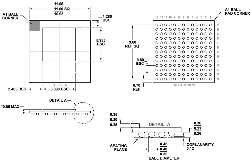
\*COMPLIANT TO JEDEC STANDARDS MO-275-FFAC-1 WITH THE EXCEPTION OF PACKAGE HEIGHT AND THICKNESS.
