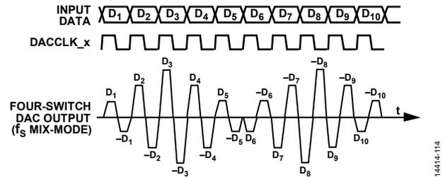
Figure 130. Mix-Mode Waveform
