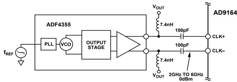
Figure 135. Possible Signal Chain for CLK± Input
