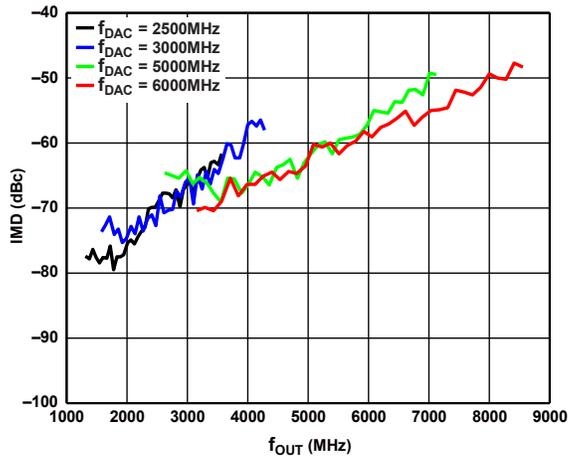
Figure 53. IMD vs.  $f_{OUT}$  over  $f_{DAC}$
