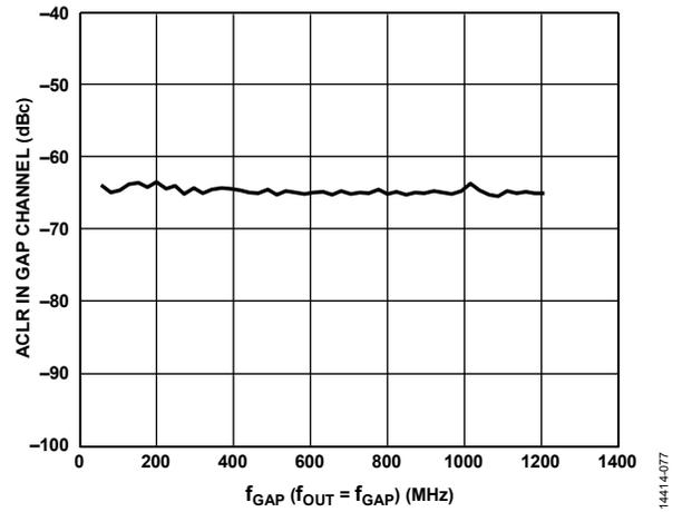
Figure 85. ACLR in Gap Channel vs.  $f_{GAP}$
