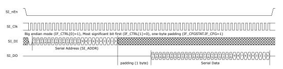
When dummy bytes are enabled (IF\_CFGSTAT.IF\_CFG), the SI slave logic enables an error check that sends out 0x88888888 and sets IF\_CFGSTAT.IF\_STAT if the SI master does not provide enough time for register read.
