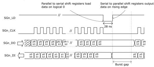
The SGPIO values are output in bursts followed by assertion of the SGn\_LD signal. Values can be output as a single burst or as continuous bursts separated by a configurable burst gap. The maximum length of a burst is 32 × 4 data cycles. The burst gap is configurable in steps through SIO\_CFG.SIO\_BURST\_GAP\_DIS, SIO\_CFG.SIO\_BURST\_GAP, and SIO\_CFG.SIO\_REDUCED\_GAP.
