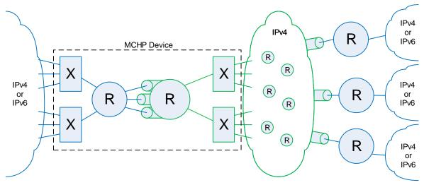
The frames forwarded between the blue and the green routers are pure IP packets, i.e. they have no associated Ethernet protocol layer including no associated VLAN or ingress port number.
