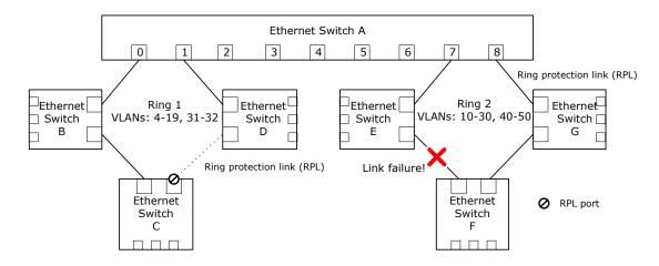
To avoid having to perform write access to the VLAN\_PORT\_MASKs of each of VID 10–30 and 40–50, VLAN TUPE can be used instead. The following table lists the VLAN TUPE parameters to reconfigure the VLAN table.
