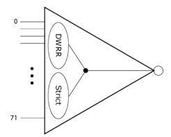
The lower indexes are arbitrated in the effort to achieve a bandwidth ratio between them. In this regard, the bandwidth can be measured in frames, data bits, or line bits (including IFG). Each input is configured with a cost setting, and the algorithm strives to give n times more bandwidth to input A than B, if the cost configuration for A is n times lower than B.
