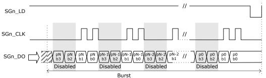
The frequency of the SGn\_CLK clock output is configured through SIO\_CLOCK.SIO\_CLK\_FREQ. The SGn\_LD output is asserted after each burst; this output is asserted for a period of 25 ns to 30 ns. The polarity of SGn\_LD is configurable through SIO\_CFG.SIO\_LD\_POLARITY.
