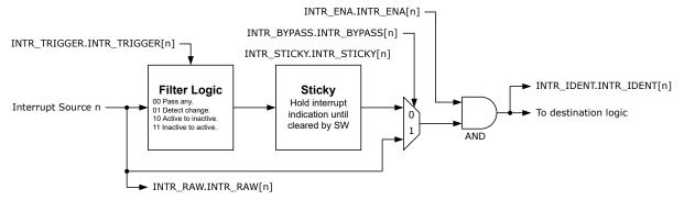
The current value of an interrupt source is available in INTR\_RAW.INTR\_RAW[n]. INTR\_STICKY.INTR\_STICKY[n] is set when the interrupt controller detects an interrupt. There are following detection methods.
