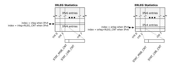
Each counter type must be configured to count either bytes or frames. (ANA\_AC:STAT\_GLOBAL\_CFG\_IRLEG: STAT\_GLOBAL\_CFG.CFG\_CNT\_BYTE and ANA\_AC:STAT\_GLOBAL\_CFG\_ERLEG: STAT\_GLOBAL\_CFG.CFG\_CNT\_BYTE)
