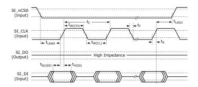
Figure 7-7. SI Output Data Timing Diagram for Slave Mode
