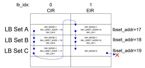
If only MEF 10.2 bandwidth profiles are required, then the LB Set must be configured as shown in the following figure.
