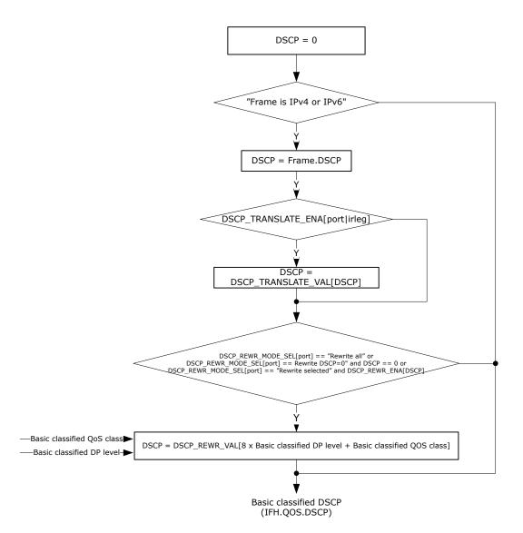
Note that the DSCP translation part is common for both QoS, DP, and DSCP classification, and the DSCP trust part is common for both QoS and DP classification.
