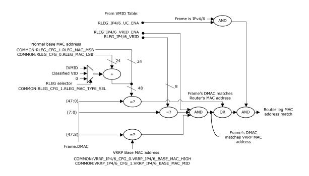
The packet is a candidate for unicast routing if a frame's DMAC matches one of the router leg MAC addresses. Packets sent to the router itself will also match the router leg MAC address, but these will be caught through entries in the ARP table.
