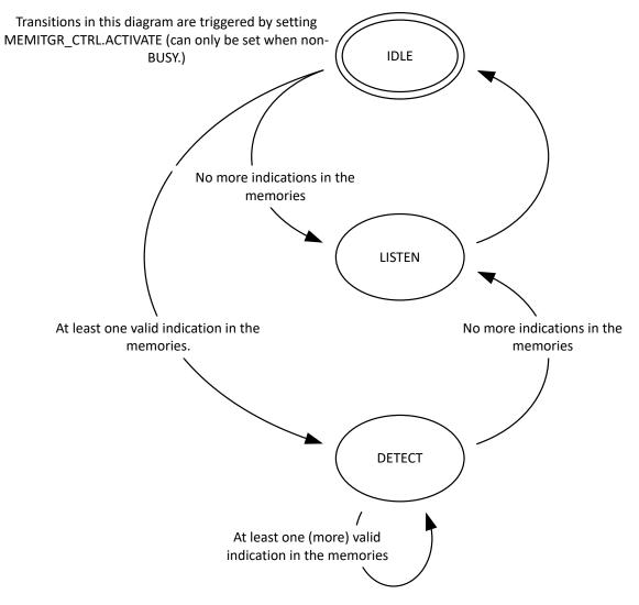
The first time after reset that MEMITGR\_CTRL.ACTIVATE is set, the monitor resets the detection logic in all the memories and transitions directly from IDLE to LISTEN state.
