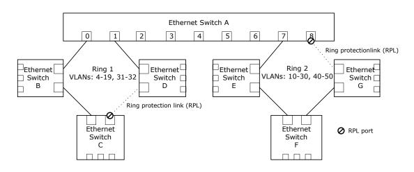
The following table shows the configuration of the VLAN table of switch A. The VLAN\_PORT\_MASK bit shows only the value for the ring ports. For the other ports (ports 2-6), the VLAN\_PORT\_MASK bits are assumed to be 0.
