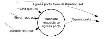
The CPUQ field instructs which of the eight CPU extraction queues should get a copy of this frame. Each queue in the queue system is translated into either one of the two internal CPU ports or to a front port. The egress QoS class can be set to the same value as the ingress QoS class or to a specific value per CPU extraction queue. A super priority can also be used. For more information, see 4.26.9.2 Super Priorities.
