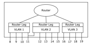
Within the device, a router leg is identified by a 9-bit VMID value. When a packet is being routed, it is then received by the router entity using a router leg identified by an ingress VMID (or IVMID) and transmitted on an egress router leg identified by an egress VMID (or EVMID).
