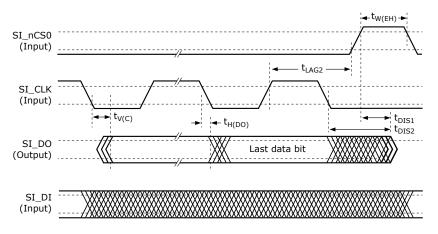
All SI signals comply with the specifications shown in the following table. The SI input timing requirements are requested at the pins of the devices.
