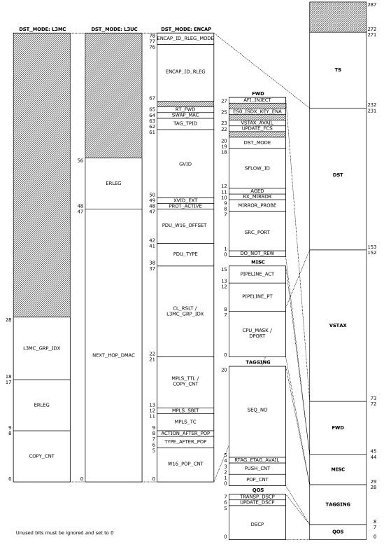
The following table shows the internal frame header fields, including information whether a field is relevant for injection, extraction, or both.
