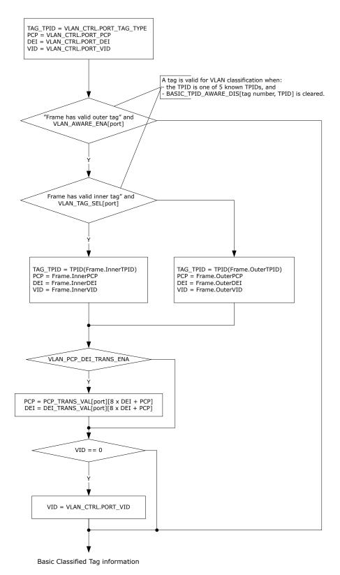
In addition to the classification shown, the port decides the number of VLAN tags to pop at egress (VLAN\_CTRL2.VLAN\_POP\_CNT) and to push at egress (VLAN\_CTRL2.VLAN\_PUSH\_CNT).
