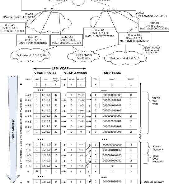
Ports o, n, and m are connected to Router A3, Host A1, and Host A2. These stations are included in an IP subnet associated with VLAN 1 and connected to the router by router leg 1. Router leg 1's MAC address is shown.
