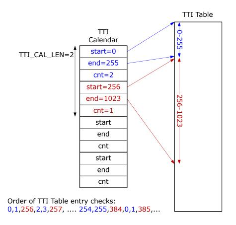
In the example, it takes  $(256/2) \times (1 + 2) \times 4 = 1536$  clock cycles to service all TTIs in the blue section. With a clock cycle for instance 4 ns, the TTIs in the blue section must not use ticks faster than  $1536 \times 4 = 6144$  ns.
