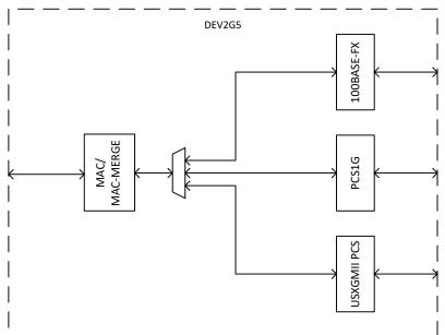
Each of the DEV5G, DEV10G, and DEV25G Port modules have an associated DEV2G5 port module as a shadow device to handle speeds less than or equal to 2.5G.
