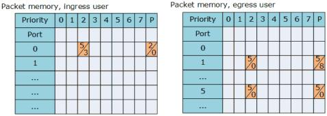
For PFC purposes, the congestion controller contains an additional accounting sheet of the ingress memory consumption. The sheet has its own set of thresholds. The result of the accounting is whether to send PFC pause frames towards the link partner.
