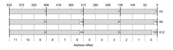
In total, X3 entries require 1 type-group bits per entry, X6 entries require 3 type-group bits per entry, and X12 entries require 7 type-group bits per entry.
