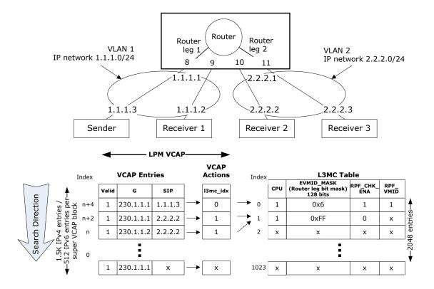
A sender host with IPv4 address 1.1.1.3 is transmitting IPv4 multicast frames to the group address 230.1.1.1 and DMAC = 0x01005E010101. The frames must be L2 forwarded to receivers in VLAN 1 and L3 forwarded to receivers in VLAN 2. For the latter, an entry for the (1.1.1.3, 230.1.1.1) pair is added to the VCAP LPM.
