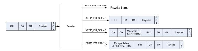
Note that for KEEP\_IFH\_SEL = 1, the frames transmitted on external ports are not valid Ethernet frames, because the extraction IFH precedes the DMAC. This format cannot be used for forwarding to a standard Ethernet device. The CPU ports, VD0 and VD1 keep the IFH and use KEEP\_IFH\_SEL = 1.
