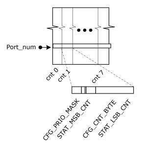
Before using the statistic counters, they must be initialized to clear all counter values and sticky bits (ANA\_AC:STAT\_GLOBAL\_CFG\_PORT:STAT\_RESET.RESET).
