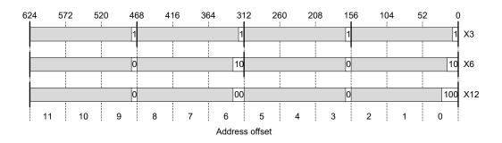
In total, X3 entries require one type-group bits per entry, X6 entries require three type-group bits per entry, and X12 entries require 7 type-group bits per entry.
