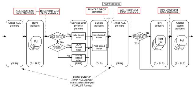
At most, each frame can see one ACL policer. ACL policing can occur as either outer or inner ACL-based. VCAP IS2 action IS\_INNER\_ACL allows ACL policing to occur before or after service DLB policing and service statistics.
