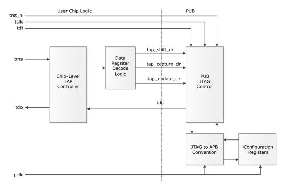
A (2 + g + 32)-bit data register is used to create read/write transactions on the configuration port; g is the width of the configuration port address. The JTAG instruction register is not supported. This also means that no JTAG instructions are supported.
