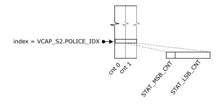
Each counter type must be configured whether bytes or frames are counted (ANA\_AC:STAT\_GLOBAL\_CFG\_ACL: STAT\_GLOBAL\_CFG.CFG\_CNT\_BYTE).
