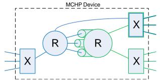
In order to have the device route the frame twice (once for the blue IP domain and once for the green IP domain), the frame must be processed twice by ANA-QSYS-REW.
