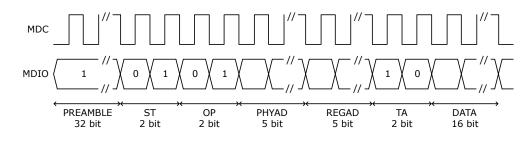
A read transaction is done in a similar way. First, read the DATA\_REG0 and then read the DATA\_REG1. As with a write operation, the switch core register read is not initiated before the DATA\_REG1 register is read. In other words, the returned read value is from the previous read transaction.
