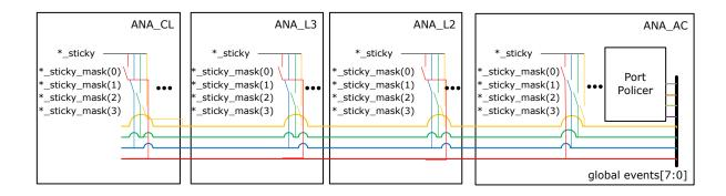
The global events [3:0] are typically allocated for detected control frames, frames dropped due to wrong configuration, frames dropped due to VLAN filtering, and so on.
