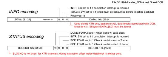
As mentioned before, the amount of data blocks that can be associated to a DCB is configurable. Moreover, a DCB does not have to use all of them. The FDMA processes the data-block related fields of a DCB in-order, and terminates the processing of a DCB when an invalid data-block field is encountered or when the end of the DCB is reached. For extraction DCBs, a data-block field is invalid if the data-block pointer is not 64-bit aligned. For injection DCBs, a data-block length is set to zero.
