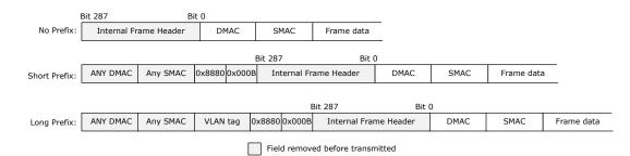
Frames are injected without prefix from internal CPU or directly attached CPU.
