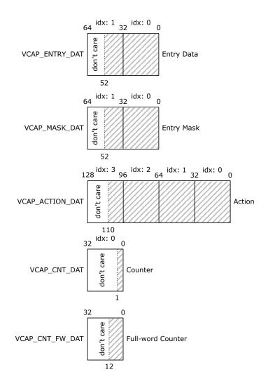
Entries have both entry data and entry mask fields. This allows a don't-care of any bit position in the key when matching a key against entries.
