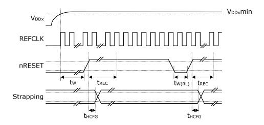
The signal applied to the nRESET input must comply with the specifications listed in the following table at the reset pin of the devices.
