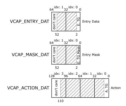
When programming the entry's type-group field, the mask bits must be set to zeros, so that the typegroup bits consist of match-1 or match-0, or both.
