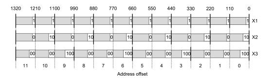
In total, X1 actions require 1 type-group bit per action, X2 actions require 3 type-group bits per action, and X3 actions require 7 type-group bits per action.
