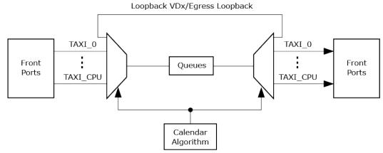
The front ports are connected to taxi busses and must be guaranteed bandwidth corresponding to their line speed.
