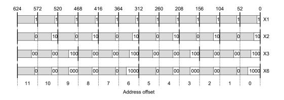
In total, X1 entries require 1 type-group bit per entry, X2 entries require 3 type-group bits per entry, X3 entries require 7 type-group bits per entry, and X6 entries require 13 type-group bits per entry.
