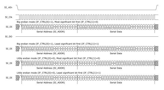
When reading registers using the SI interface, the device needs to prepare read data after receiving the last address bit. The access time of the register that is read must be satisfied before shifting out the first bit of read data. For information about access time, see 5.5.1 Register Access and Multimaster Systems. The external CPU must apply one of the following solutions to satisfy read access time.
