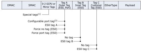
Mirror tag is controlled by REW::MIRROR\_PROBE\_CFG.REMOTE\_MIRROR\_CFG. GCPU tag is controlled by REW::GCPU\_CFG.GCPU\_TAG\_SEL.
