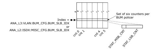
Each of the two counters in a counter set can be configured to which frames are counted and, whether bytes or frames are counted. This configuration is shared among all counter sets.
