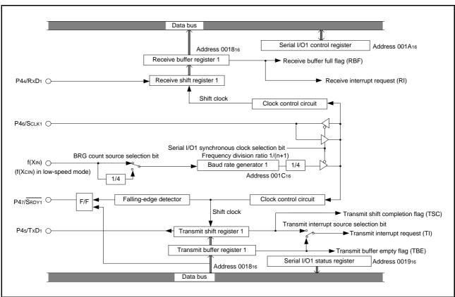
Fig 36. Block diagram of clock synchronous serial I/O1
