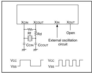
Fig 65. External clock input circuit
