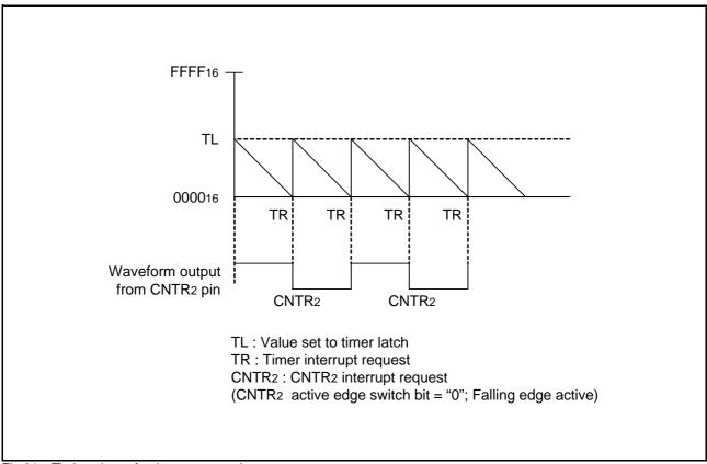
Fig 31. Timing chart of pulse output mode
