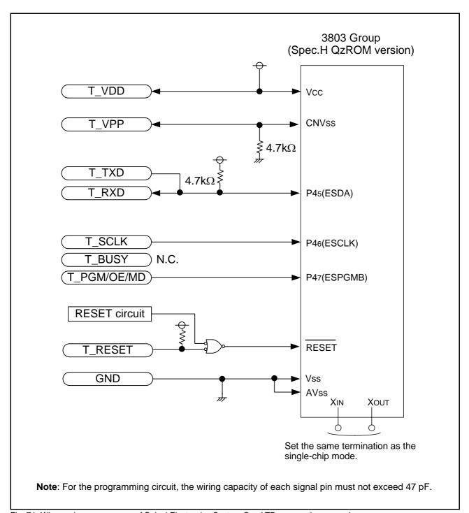
Fig. 71 When using programmer of Suisei Electronics System Co., LTD, connection example
