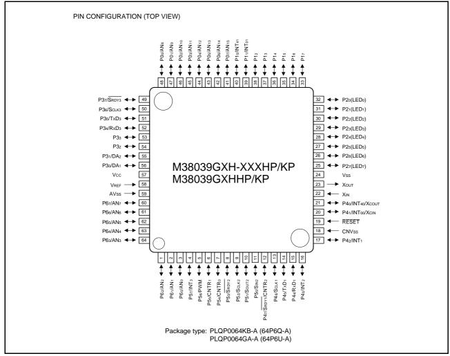
Fig 1. 3803 group (Spec.H QzROM version) pin configuration (PLQP0064KB-A/PLQP0064GA-A)
