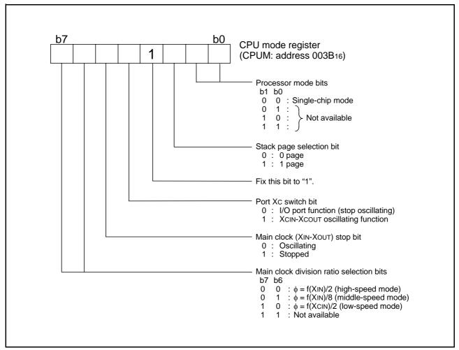
Fig 9. Structure of CPU mode register
