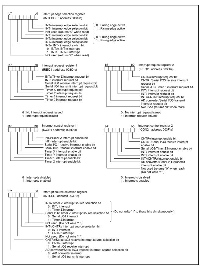
Fig 21. Structure of interrupt-related registers
