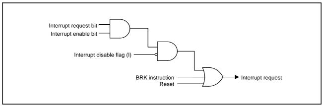
Fig 20. Interrupt control diagram
