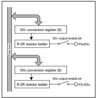
Fig 57. Block diagram of D/A converter
