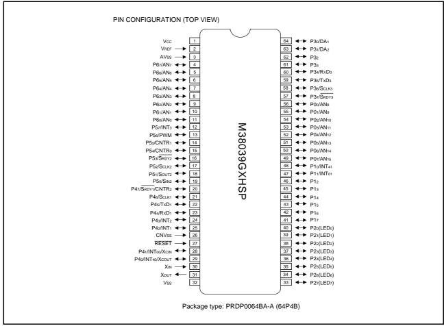
Fig 2. 3803 group (Spec.H QzROM version) pin configuration (PRDP0064BA-A)
