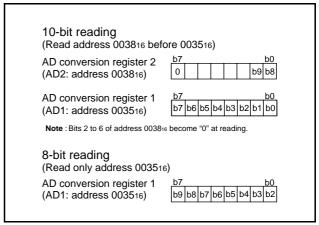
Fig 55. Structure of 10-bit A/D mode reading
