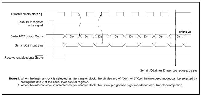
Fig 43. Timing of serial I/O2
