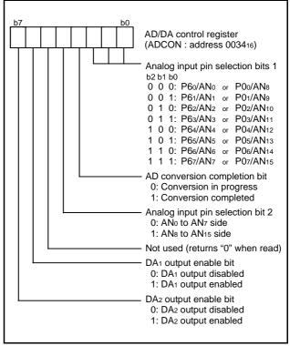
Fig 53. Structure of AD/DA control register
