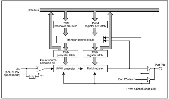
Fig 50. Block diagram of PWM function
