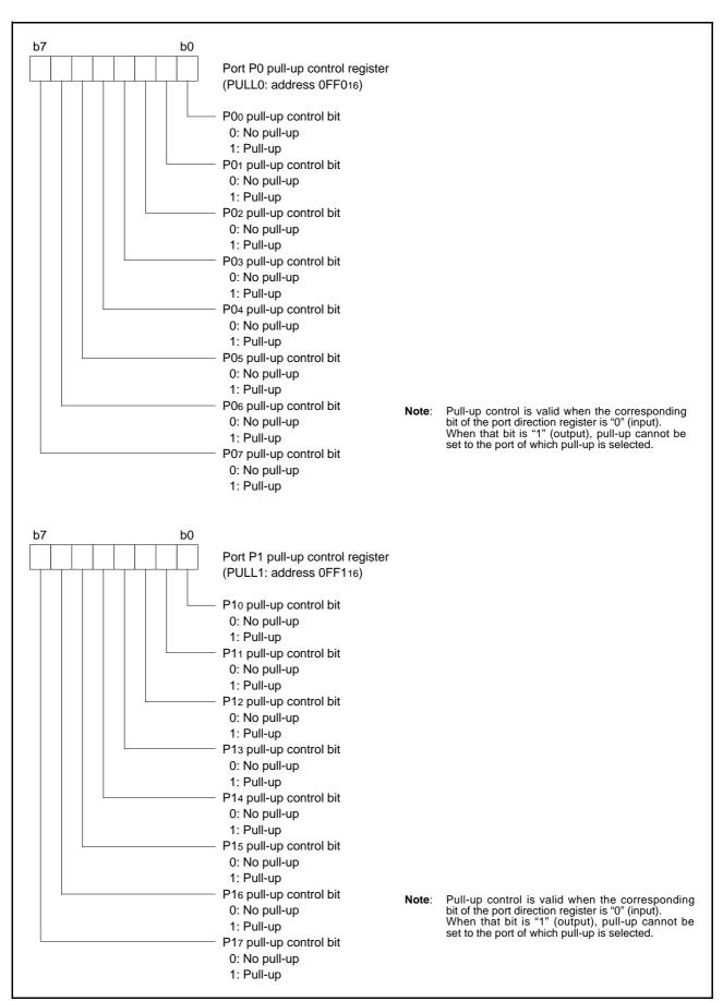
Fig 16. Structure of port pull-up control register (1)
