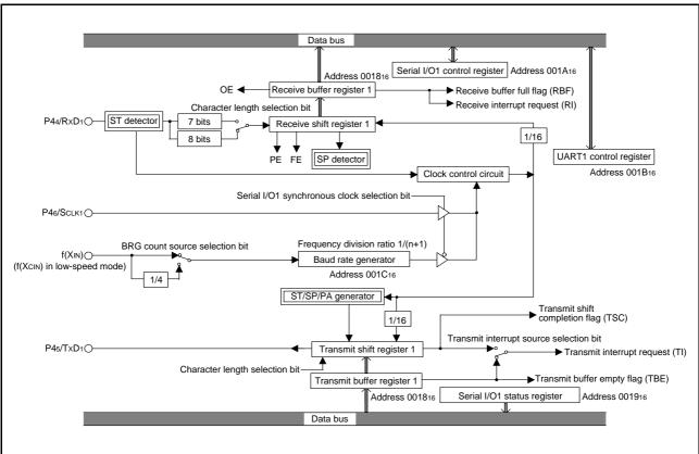
Fig 38. Block diagram of UART serial I/O1
