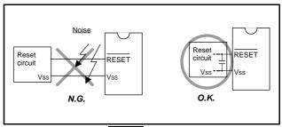
Fig. 76 Wiring for the RESET pin
