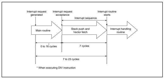
Fig 22. Time up to execution in interrupt routine
