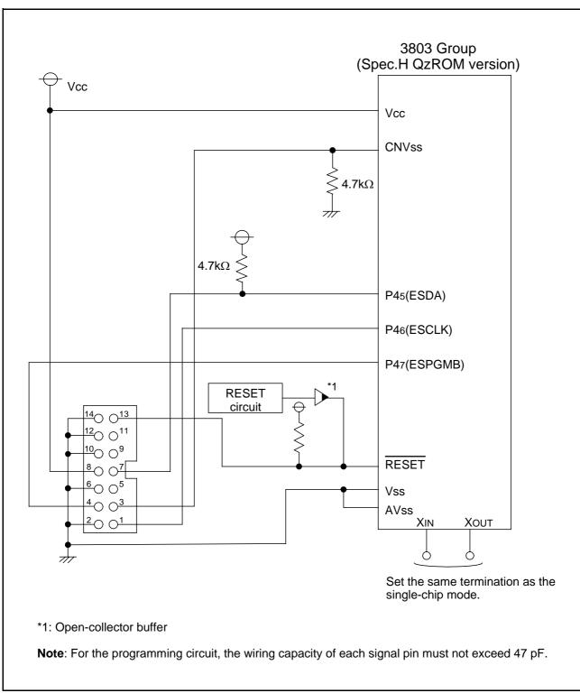
Fig. 72 When using E8 programmer connection example
