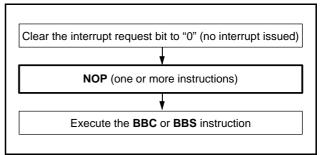
Fig 81. Sequence of check of interrupt request bit
