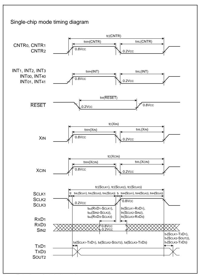
Fig 89. Timing diagram (in single-chip mode)
