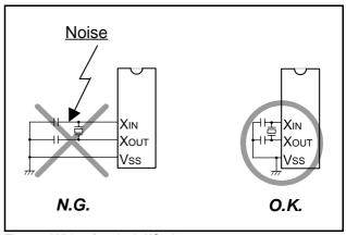
Fig. 77 Wiring for clock I/O pins
