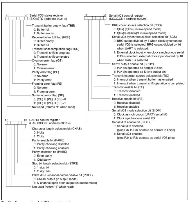
Fig 48. Structure of serial I/O3 control registers
