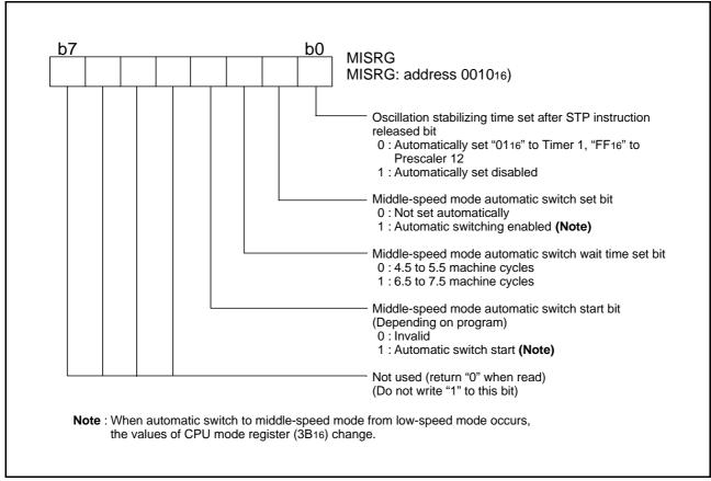
Fig 10. Structure of MISRG
