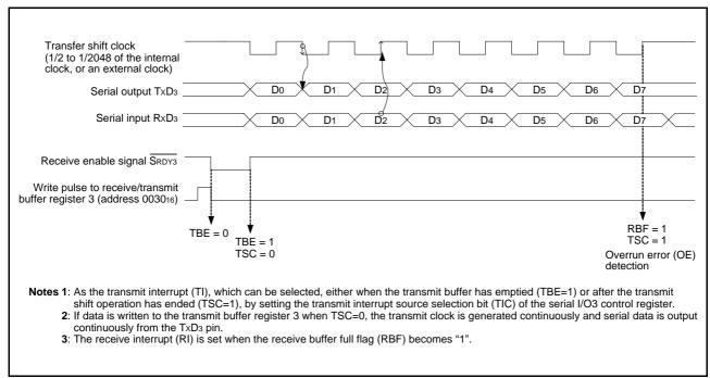
Fig 45. Operation of clock synchronous serial I/O3
