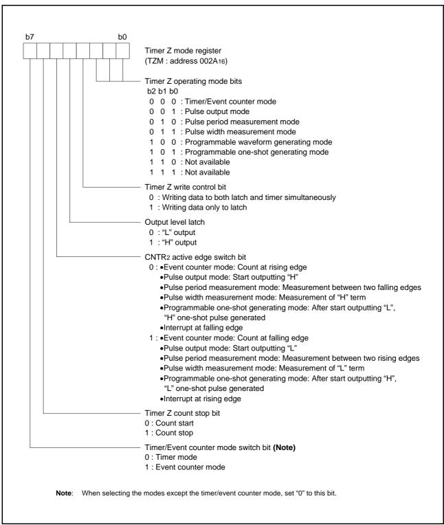
Fig 29. Structure of timer Z mode register
