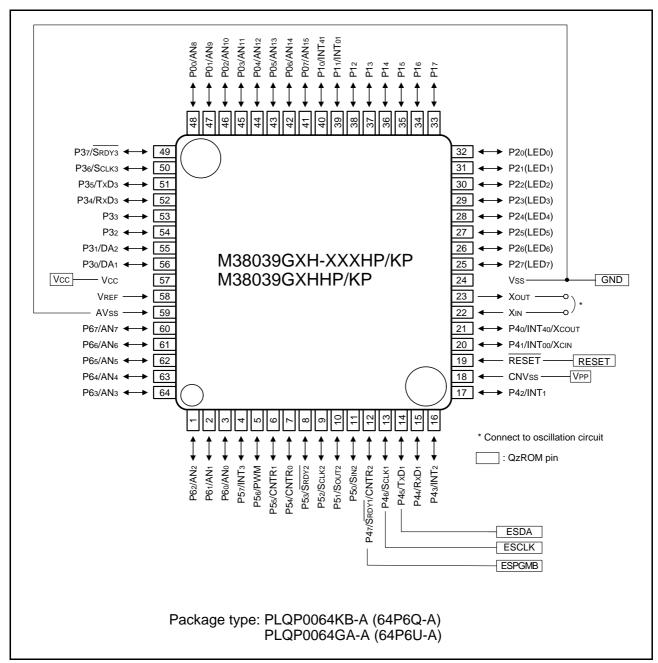
Fig. 68 Pin connection diagram (M38039GXH-XXXHP/KP, M38039GXHHP/KP)
