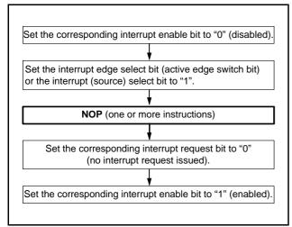
Fig 80. Sequence of changing relevant register
