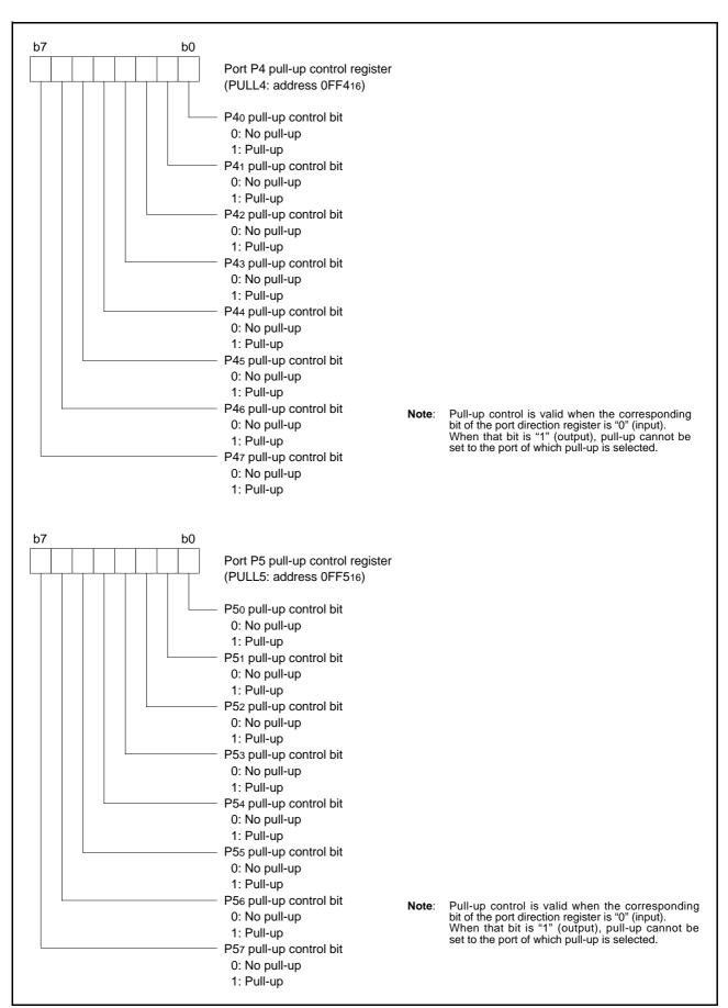
Fig 18. Structure of port pull-up control register (3)
