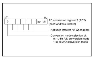
Fig 54. Structure of AD conversion register 2
