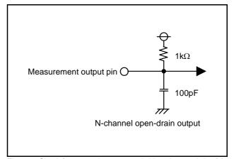
Fig 88. Circuit for measuring output switching characteristics (2)
