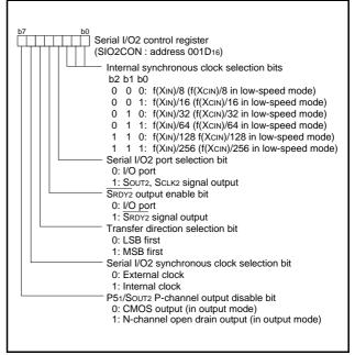
Fig 41. Structure of Serial I/O2 control register
