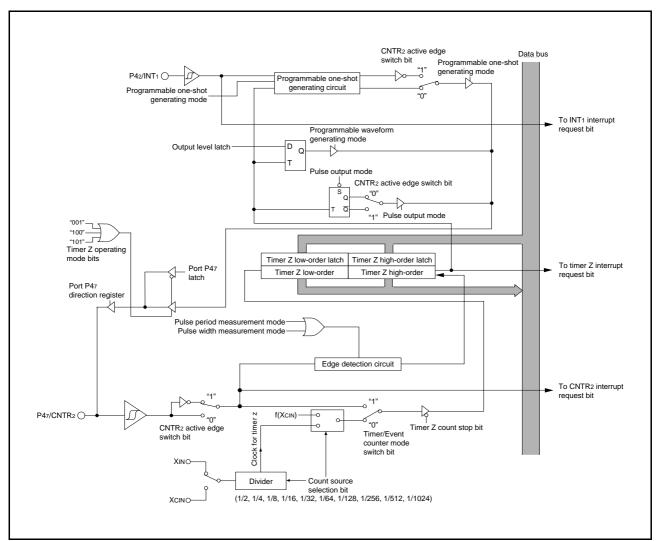
Fig 28. Block diagram of timer Z
