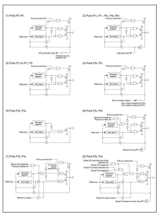
Fig 13. Port block diagram (1)
