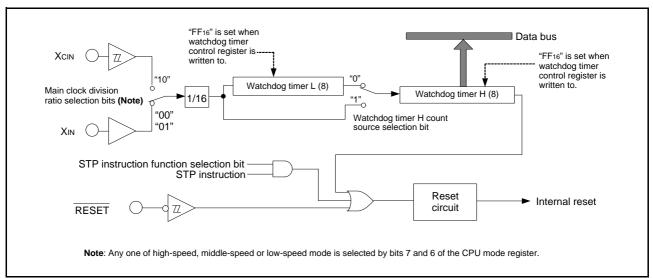
Fig 59. Block diagram of Watchdog timer
