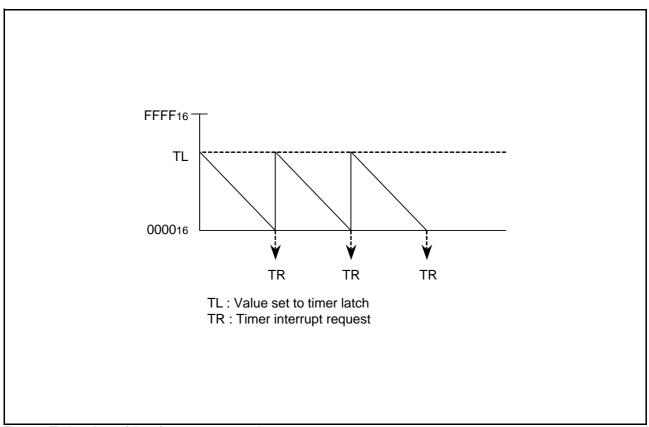
Fig 30. Timing chart of timer/event counter mode
