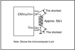
Fig 85. Wiring for the CNVss/VPP
