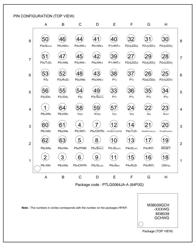
Fig 3. Pin configuration (Top view) (PTLG0064JA-A (64F0G))
