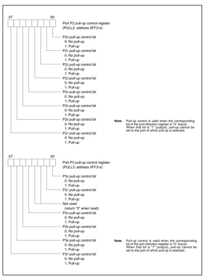
Fig 17. Structure of port pull-up control register (2)
