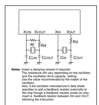
Fig 64. Ceramic resonator circuit
