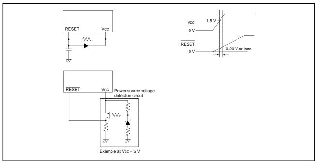
Fig 61. Reset circuit example
