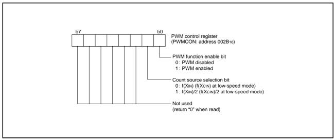
Fig 51. Structure of PWM control register
