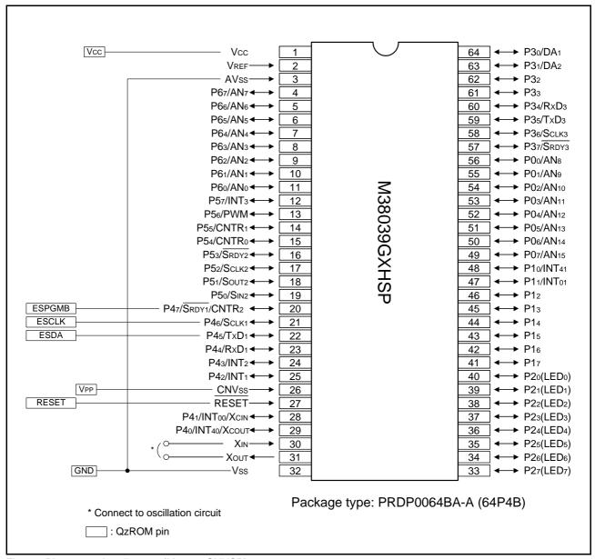
Fig. 69 Pin connection diagram (M38039GXHSP)
