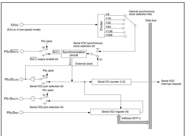
Fig 42. Block diagram of serial I/O2
