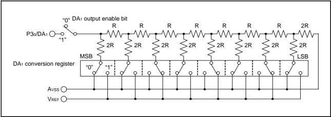
Fig 58. Equivalent connection circuit of D/A converter (DA1)
