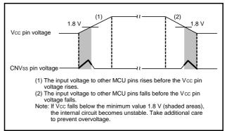
Fig 84. Timing Diagram (bold-lined periods are applicable)
