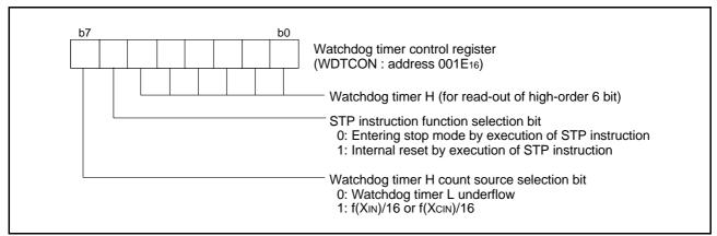
Fig 60. Structure of Watchdog timer control register
