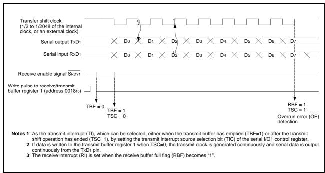
Fig 37. Operation of clock synchronous serial I/O1
