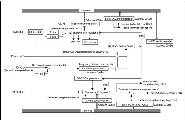
Fig 46. Block diagram of UART serial I/O3
