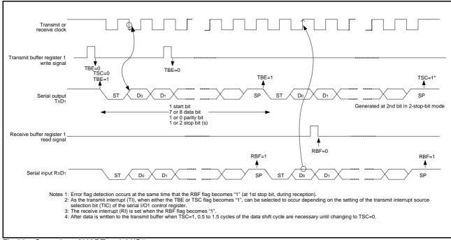
Fig 39. Operation of UART serial I/O1
