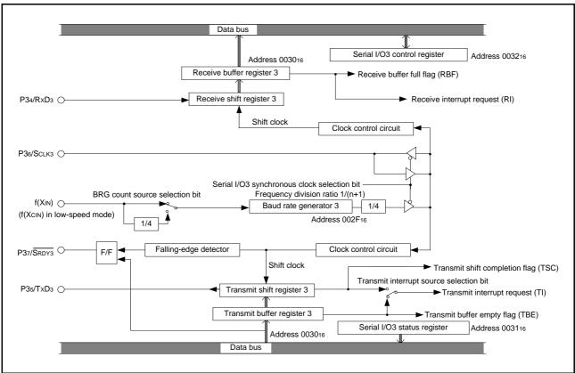
Fig 44. Block diagram of clock synchronous serial I/O3
