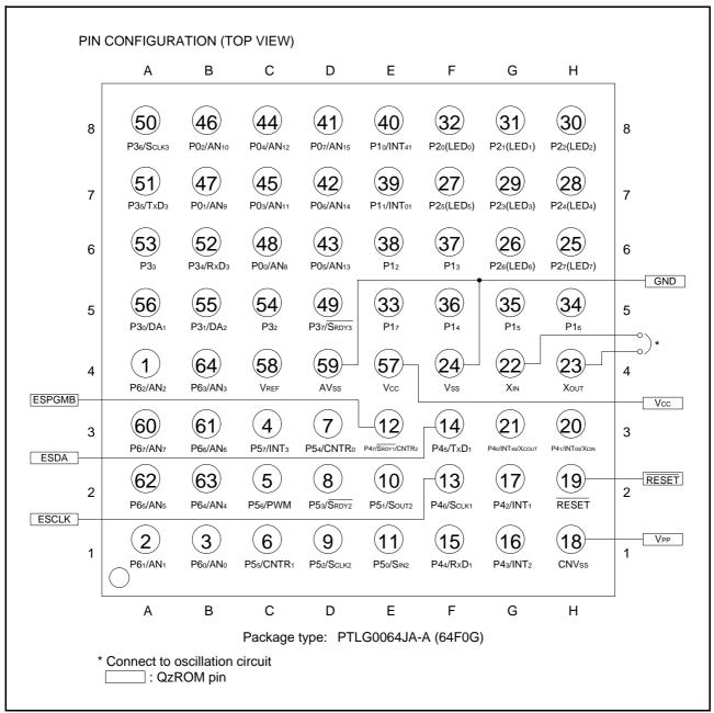
Fig. 70 Pin connection diagram (M38039GCH-XXXWG, M38039GCHWG)
