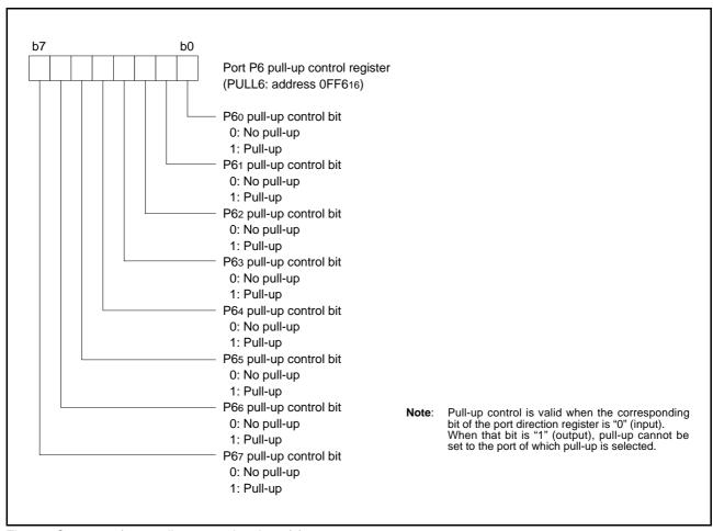
Fig 19. Structure of port pull-up control register (4)
