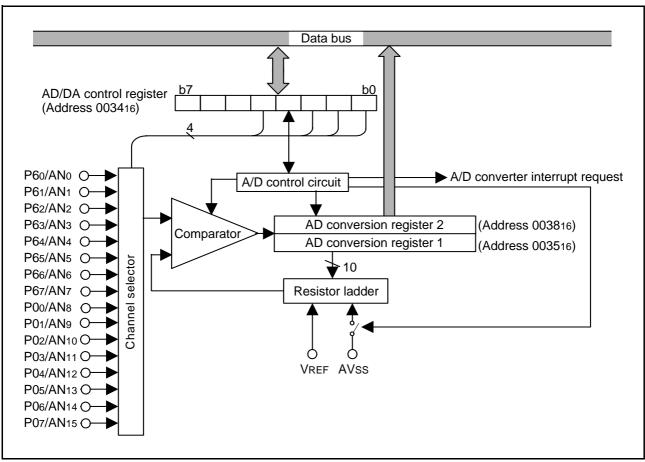
Fig 56. Block diagram of A/D converter
