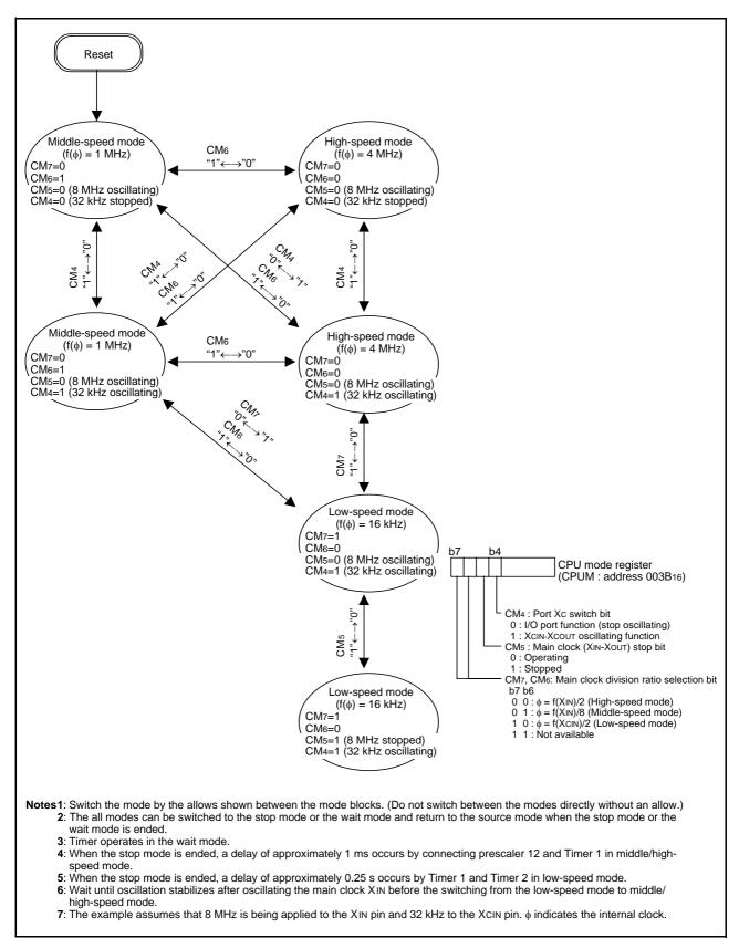
Fig 67. State transitions of system clock
