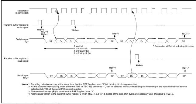
Fig 47. Operation of UART serial I/O3
