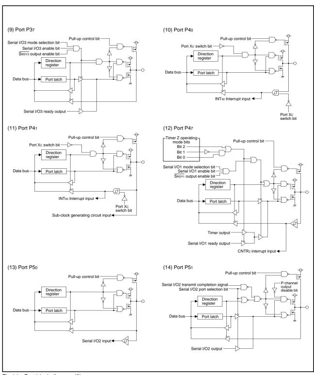
Fig 14. Port block diagram (2)
