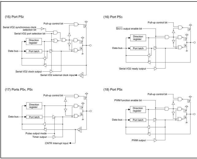
Fig 15. Port block diagram (3)
