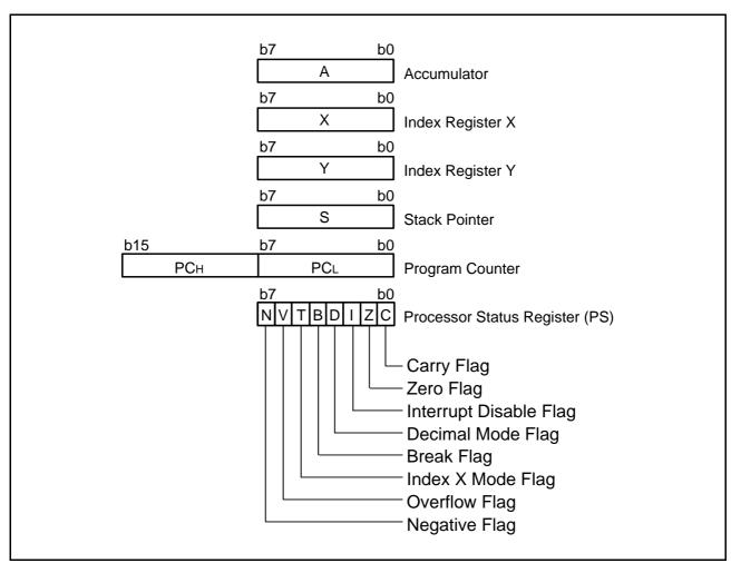
Fig 7. 740 Family CPU register structure
