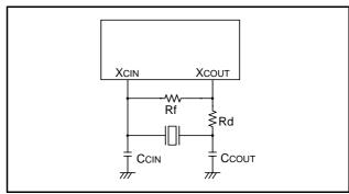
Fig 83. Ceramic resonator circuit
