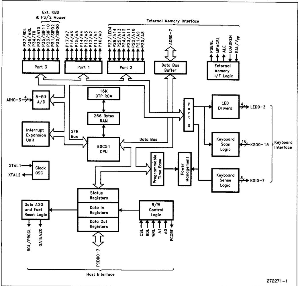
Figure 1. Block Diagram
