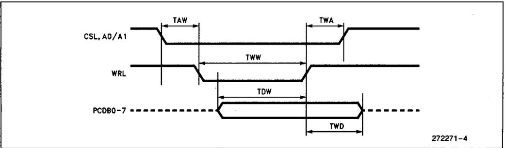
Figure 4. Host-Interface Write
