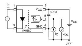
Fig. 12.1.1 V<sub>OL</sub> Test Circuit
