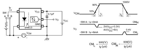
Fig. 12.1.6 Common-Mode Transient Immunity Test Circuit and Waveform
