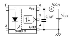
Fig. 12.1.4 I<sub>CCH</sub> Test Circuit
