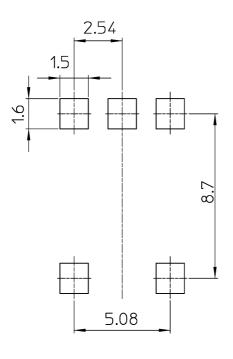
Fig. 14.1 TLP3073 Lead forming and taping option (LF1), (TP1), (LF5), (TP5)
