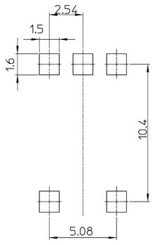
Fig. 14.2 TLP3073F Lead forming and taping option (LF4), (TP4)
