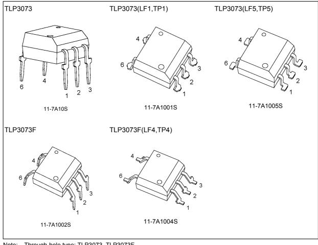
Note: Through-hole type: TLP3073, TLP3073F Lead forming option: (LF1), (LF4), (LF5) Taping option: (TP1), (TP4), (TP5)
