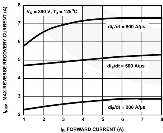
Figure 5. Maximum Reverse Recovery Current vs Forward Current
