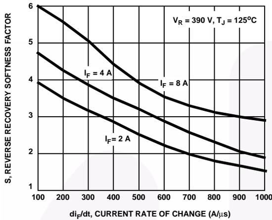
Figure 7. Reverse Recovery Softness Factor vs  $di_F/dt$
