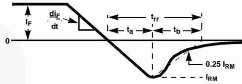
**Figure 13.  $t_{rr}$  Waveforms and Definitions**
