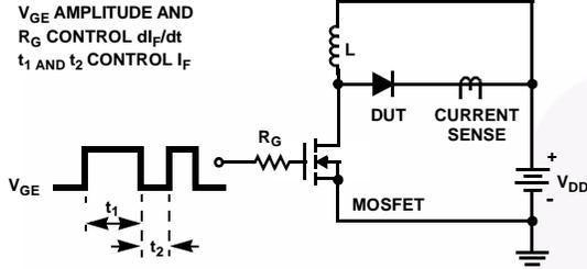
**Figure 12.  $t_{rr}$  Test Circuit**
