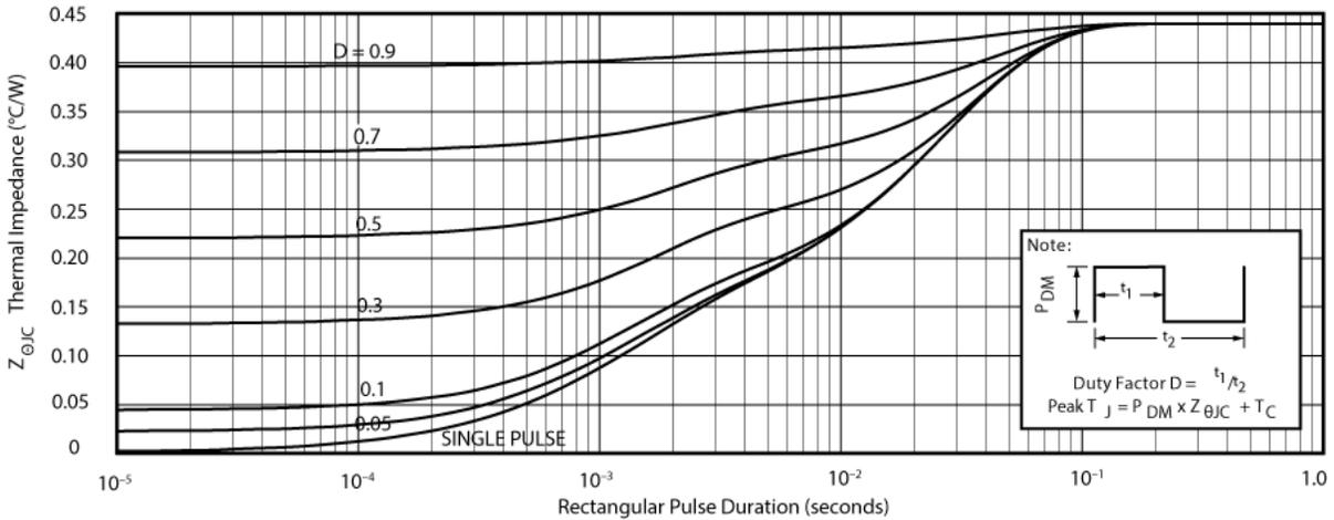
**Figure 2 • Transient Thermal Impedance Model**
