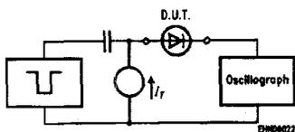
Pulse generator:  $t_p = 5\text{ }\mu\text{s}$ ,  $D = 0.05$
