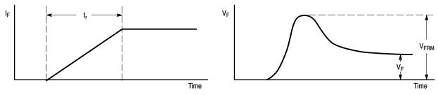
Figure 4. Peak Forward Recovery Voltage Definition
