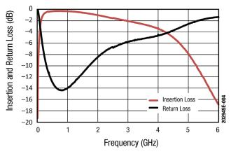
**Figure 4. Small Signal Performance without External Tuning**
