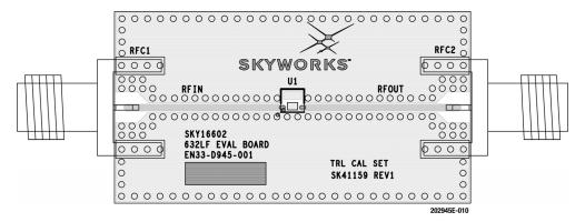
Figure 9. SKY16602-632LF Evaluation Board Assembly Diagram
