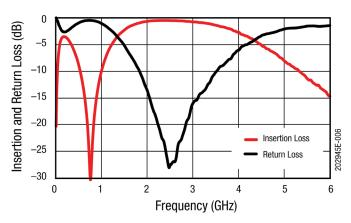
Figure 6. Small Signal Performance with External Tuning Networks Optimized for 2.45 GHz
