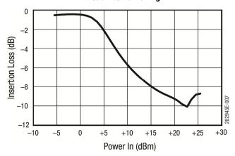
Figure 7. Insertion Loss vs CW Input Power at 2.45 GHz (Tuned Circuit)
