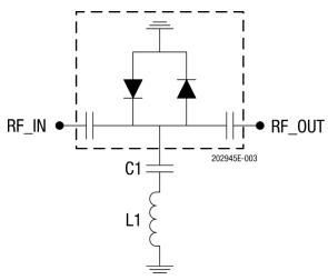
Figure 3. SKY16602-632LF Schematic with External Tuning Networks Optimized for 2.45 GHz
