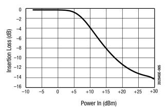
Figure 5. Insertion Loss vs CW Input Power at 0.90 GHz without External Tuning
