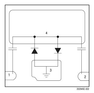
Figure 2. SKY16602-632LF Pinout (Top View)
