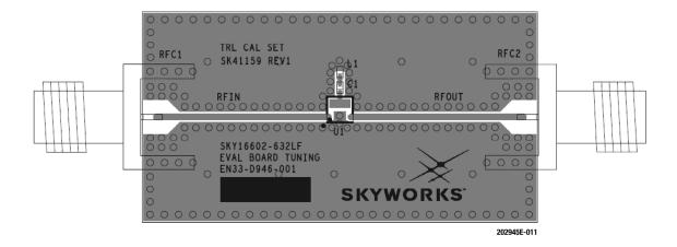
Figure 10. SKY16602-632LF Evaluation Board Assembly Diagram (Tuned Circuit)
