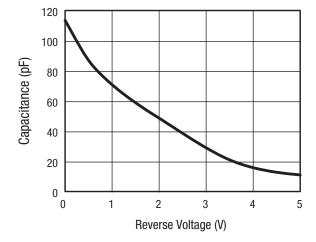
Figure 1. Capacitance vs Voltage
