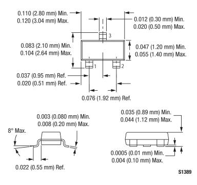
**Figure 4. SOT-23 Package Dimension Drawing**
