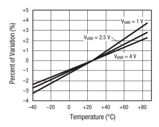
Figure 2. Relative Capacitance Change vs Temperature
