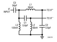
Figure 1. Example L-C IF Input Matching Network at 280MHz
