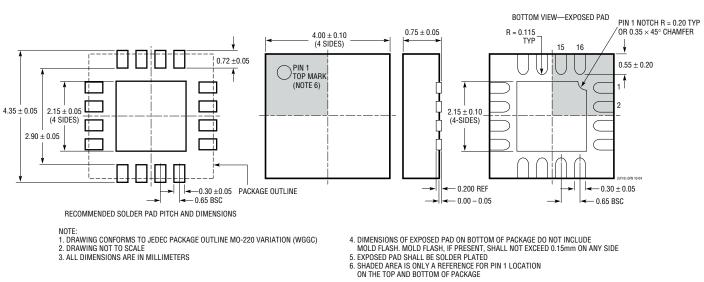
**UF Package** 16-Lead Plastic QFN (4mm  $\times$  4mm) (Reference LTC DWG # 05-08-1692)
