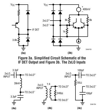
Figure 4. 2xLO Input Matching Networks for 4a) Narrow Band Tuned to 570MHz, 4b) Wide Band, 4c) Single-Ended Wide Band
