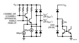
Figure 5. Simplified Circuit Schematic of I Channel (or Q Channel) Outputs and STBY (or EN) Input
