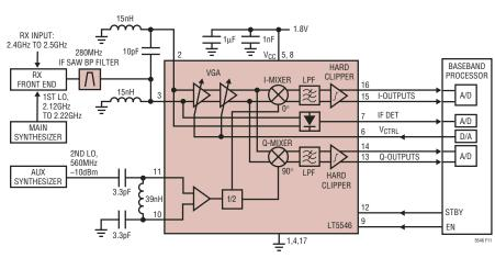
Figure 11. 2.4GHz to 2.5GHz Receiver Application (RX IF = 280MHz)
