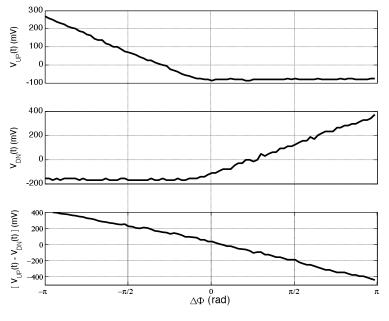
Charge pump outputs for REF lagging VCO
