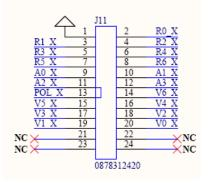
Figure 2. (J11) I/O pin configuration
