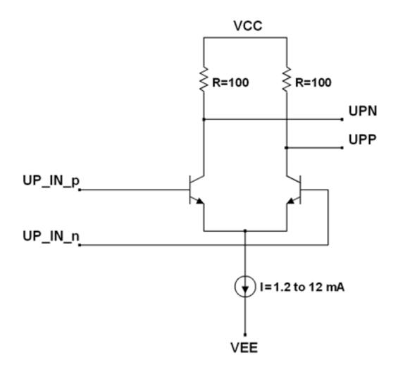
Simplified Charge Pump Output Circuit
