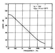
Figure 13. Common-Mode Rejection Ratio vs. Frequency
