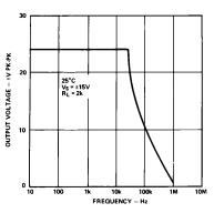
Figure 14. Large Signal Frequency Response
