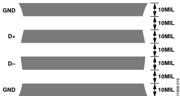
Figure 19. Arrangement of Signal Tracks
