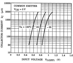
Fig. 10.3 RN1109 I<sub>C</sub>-V<sub>I(ON)</sub>
