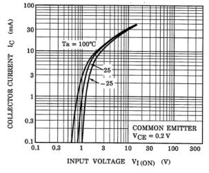
Fig. 10.1 RN1107 I<sub>C</sub>-V<sub>I(ON)</sub>
