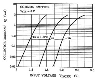
Fig. 10.5 RN1108 I<sub>C</sub>-V<sub>I(OFF)</sub>
